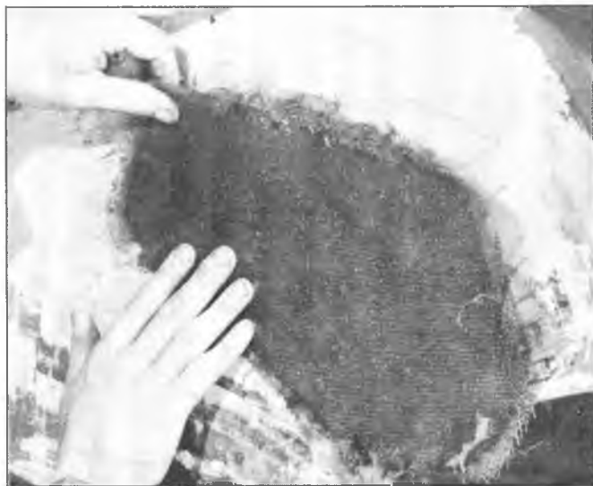
Fig. 56—Applying Laminate to Body
