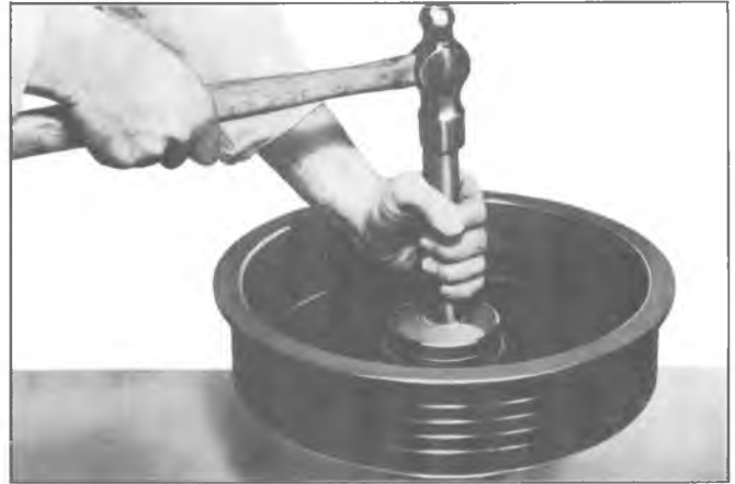
Fig. 37—Installing Hub Inner Bearing Cup (Typical)
