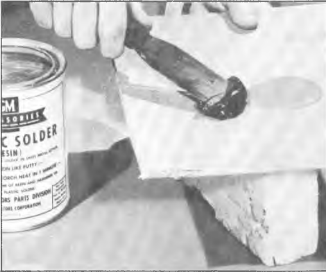
Fig. 51—Mixing Plastic Solder Material
