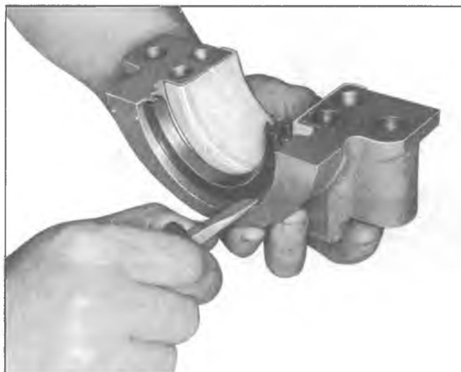
Fig. 6L—Removing Oil Seal (Lower Half) Typical
