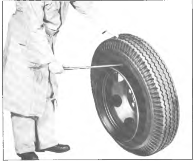
Fig. 6—Inserting Tire Iron in Second Bead
