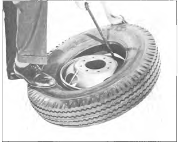
Fig. 17—Mounting First Bead
