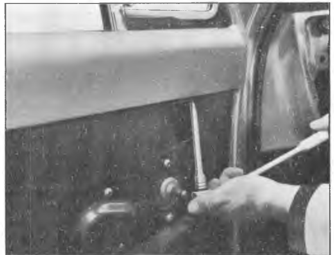
Fig. 33—Adjusting Ventilator Operating Tension
