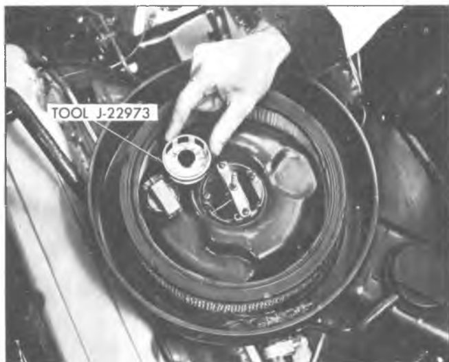
Fig. 8A—Temperature Gauge Installation
