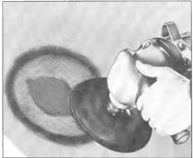
Fig. 53—Finishing Plastic Solder Repair
