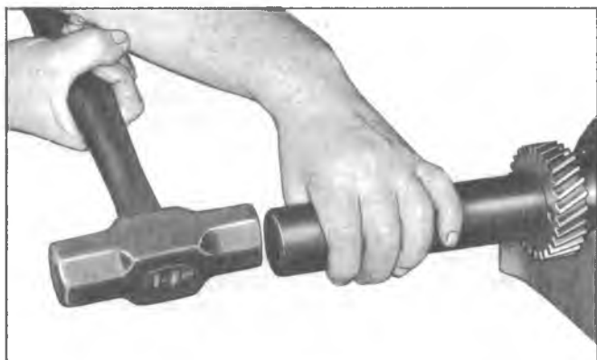
Fig. 20L—Installing Crankshaft Gear
