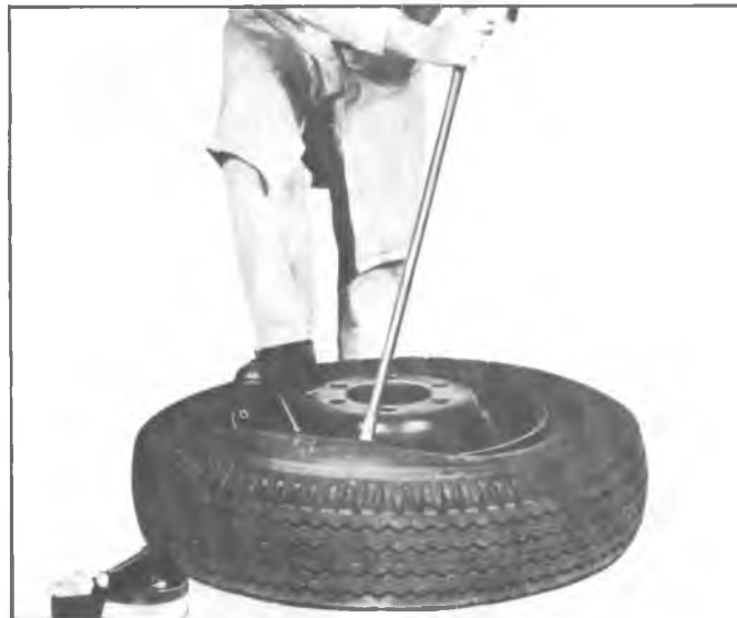
Fig. 5—Lifting Bead Over Rim
