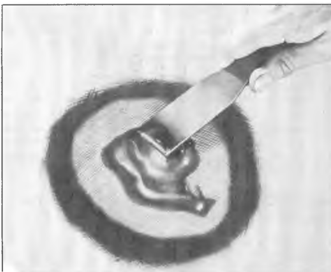
Fig. 52—Applying Plastic Solder
