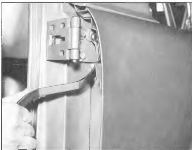
Fig. 29—Door Hinge Bolt Replacement
