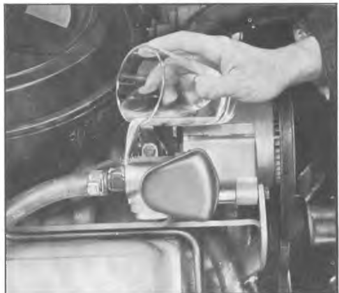
Fig. 6T-41—Checking for Leaks With a Soapy Water Solution
