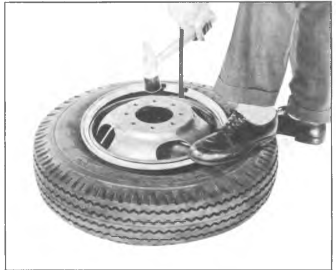
Fig. 20—Forcing Ring into Gutter
