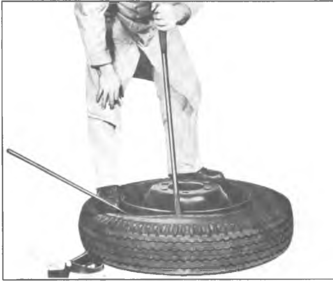
Fig. 4—Inserting Tire Iron to Lift Bead
