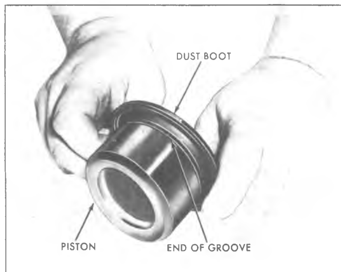
Fig. 36—Installing Boot to Piston
