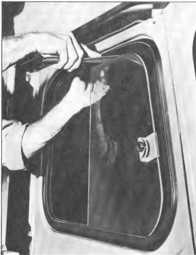
Fig. 76—Installing Sliding Glass
