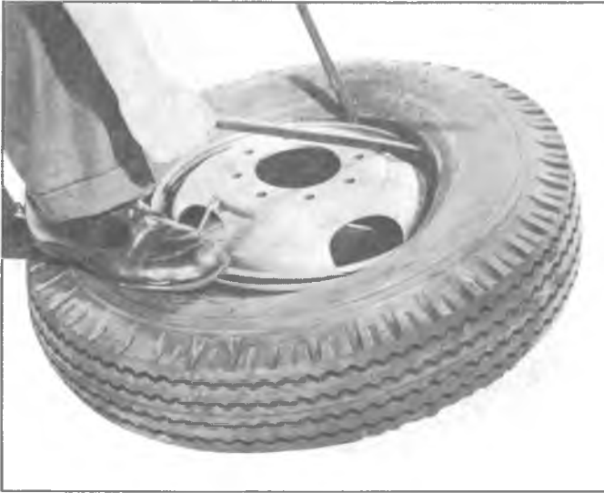
Fig. 15—Prying Bead over Edge of Rim
