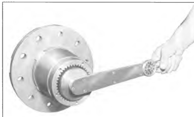
Fig. 43—Tightening Wheel Hub Bearing Adjustment Nut (Typical)
