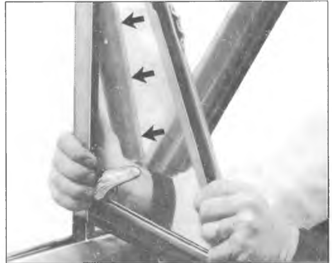
Fig. 32—Ventilator Assembly Removal
