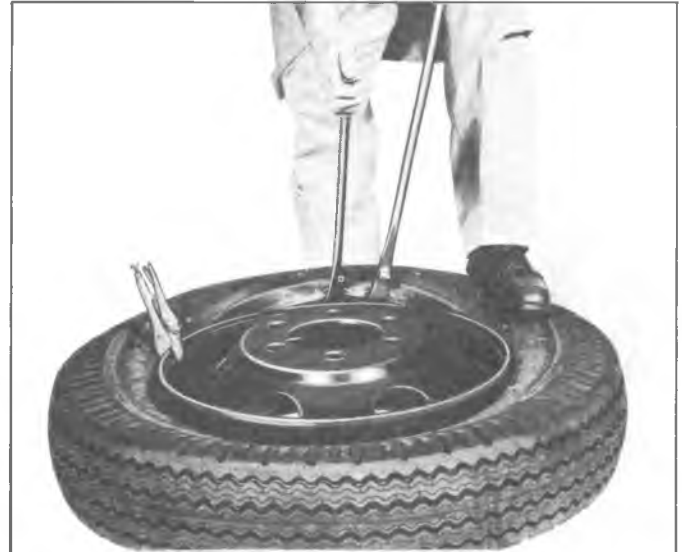
Fig. 10—Working Second Bead onto Rim
