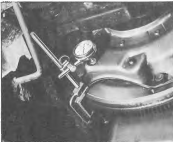
Fig. 6—Checking Pressure Plate Lift w/dial Indicator
