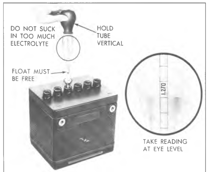
Fig. 7—Testing Specific Gravity of Battery
