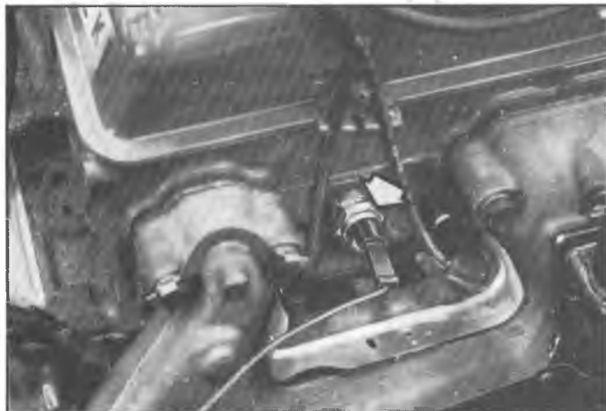
Fig. 6T-19—Small V8 Temperature Switch (Right Head)
