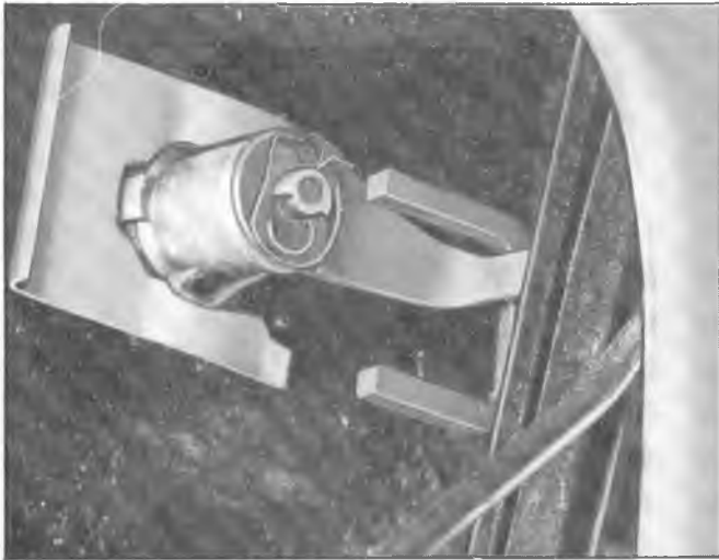
Fig. 37—Lock Cylinder Installed
