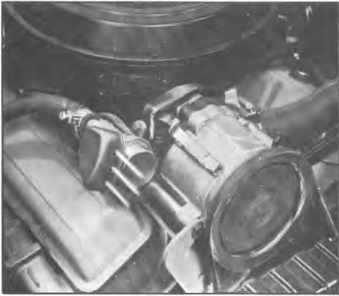
Fig. 6T-45—Momentary Blast of Air Through Diverter Valve During Engine Over Run
