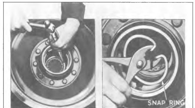
Fig. 38—Bearing Retainer Ring Removal (5200 and 7200 lb. Axle)
