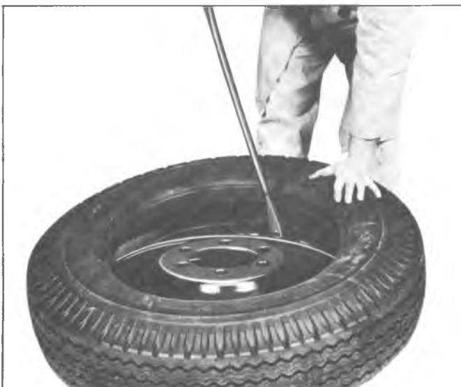
Fig. 9—Working Bead onto Rim
