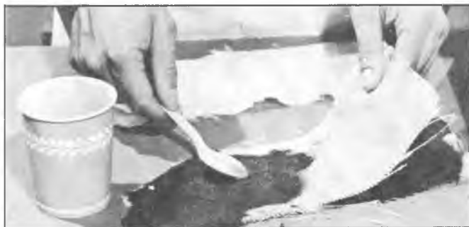
Fig. 55—Applying Resin to Fiberglass
