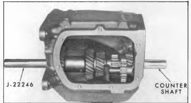
Fig. 6X--Removing Countershaft
