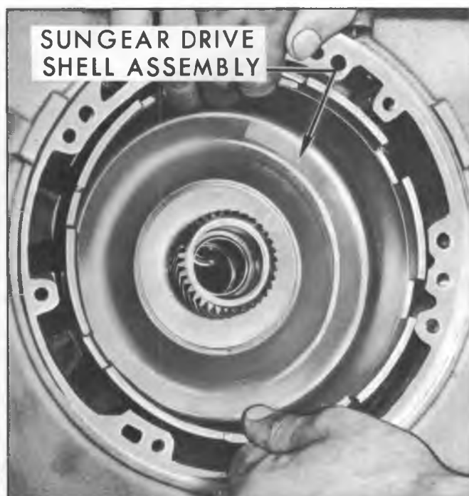
Fig. 39M--Removing Sun Gear Drive Shell
