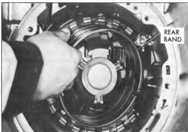
Fig. 129T--Installing Rear Band
