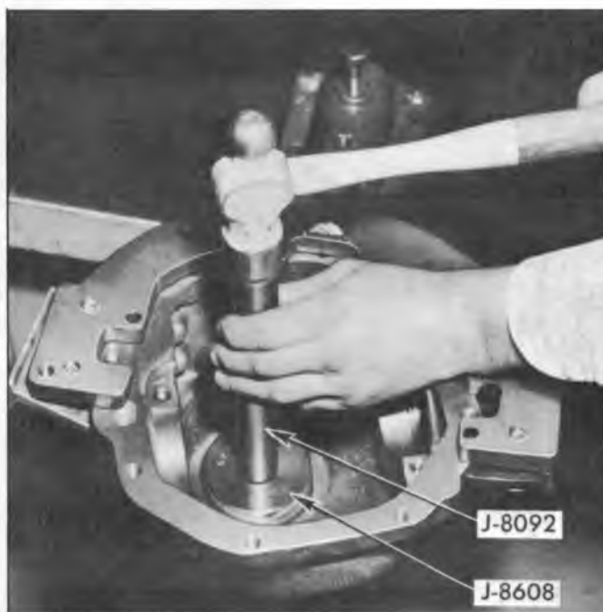
Fig. 11C--Installing Pinion Bearing Cups
