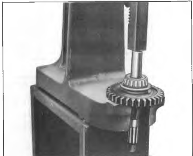
Fig. 5D--Removing Front Output Shaft Rear Bearing
