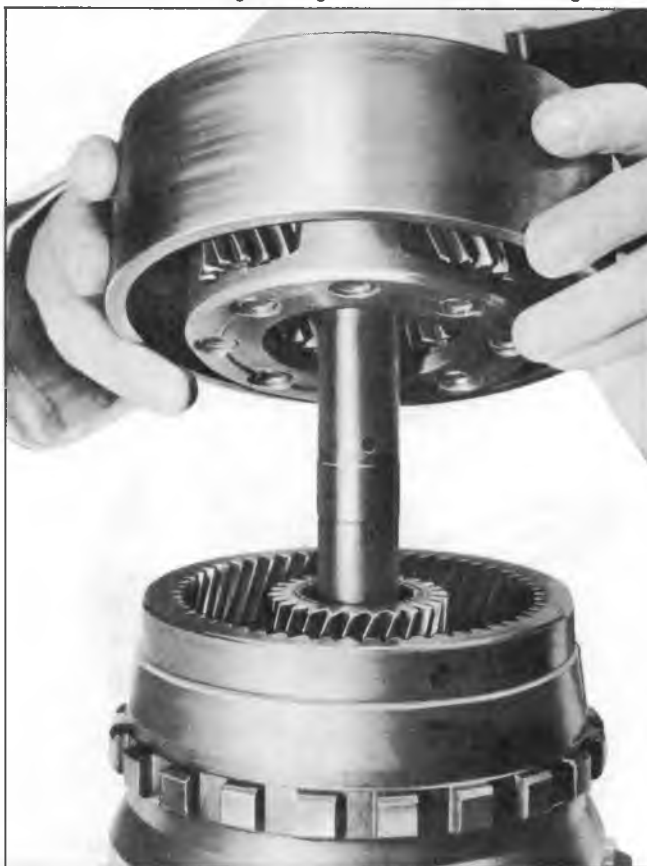
Fig. 121T--Installing Reaction Carrier
