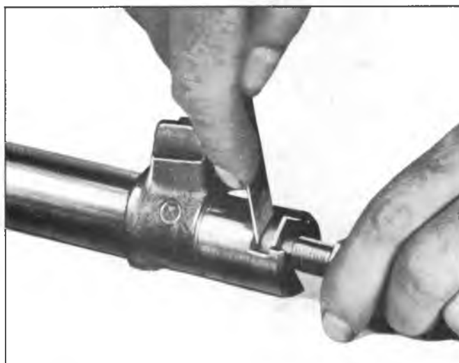
Fig. 16—Checking Lash Adjuster End Clearance
