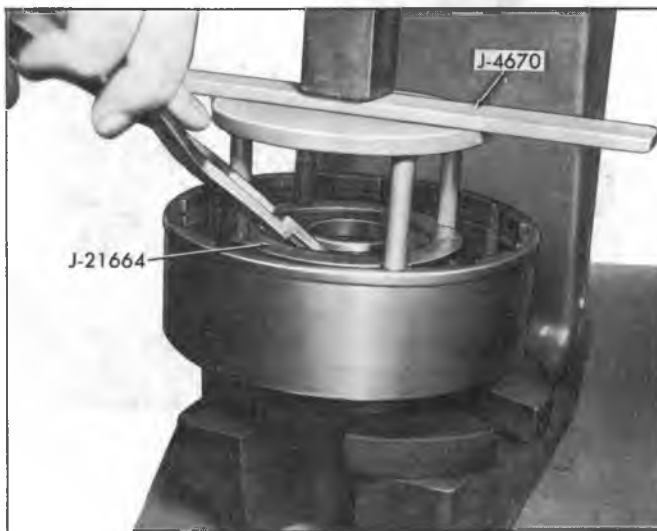
Fig. 82T--Removing or Installing Direct Clutch Snap Ring
