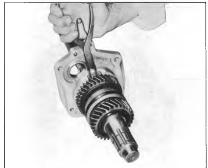
Fig. 10B—Removing Rear Bearing Retainer
