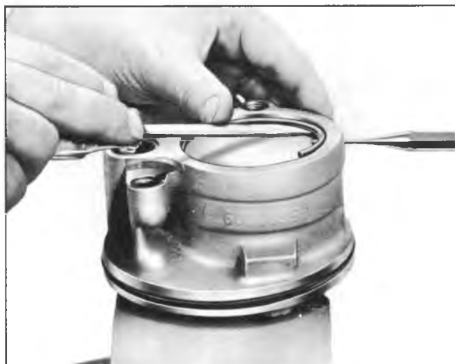
Fig. 18—Removing End Plate Ring
