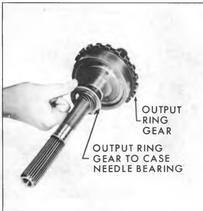
Fig. 45M--Removing Output Ring Gear to Case Needle Bearing Assembly
