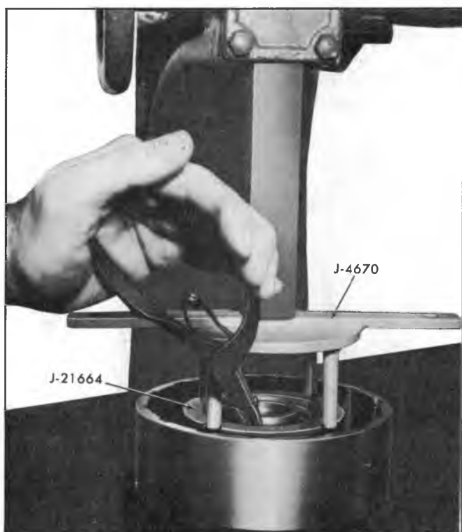
Fig. 70T--Removing Forward Clutch Spring Retaining Snap Ring
