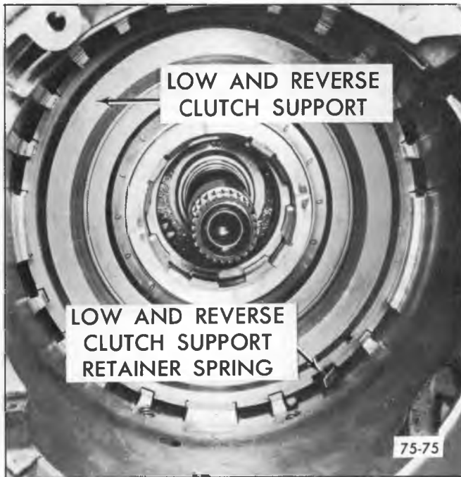
Fig. 106M--Installing Low and Reverse Clutch Support Assembly
