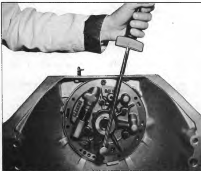
Fig. 66T--Installing Pump Cover to Pump Body
