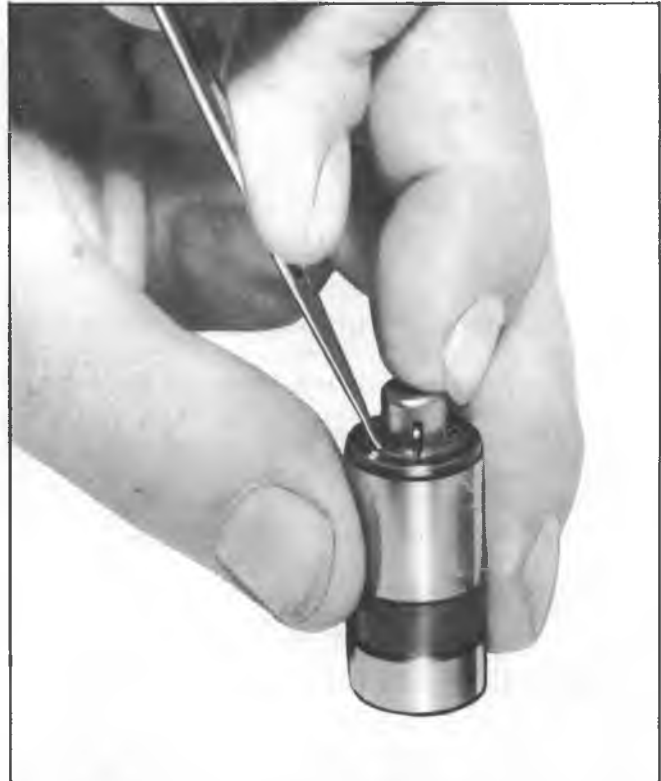
Fig. 32—Installing Ball Check Valve
