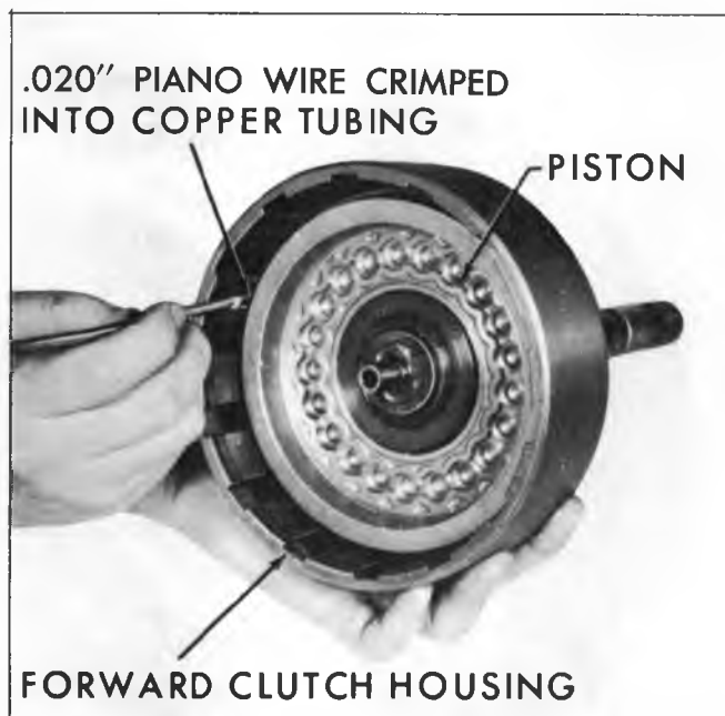
Fig. 85M--Installing Forward Clutch Piston
