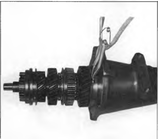
Fig. 5X--Extension to Rear Bearing Snap Ring
