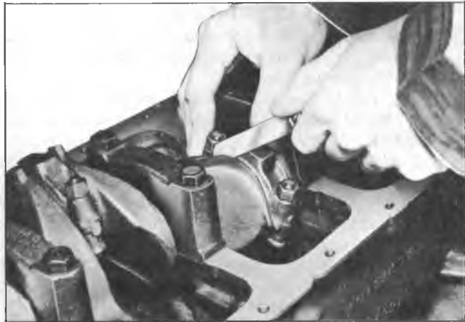
Fig. 46--Measuring Connecting Rod Side Clearance (In-Line)
