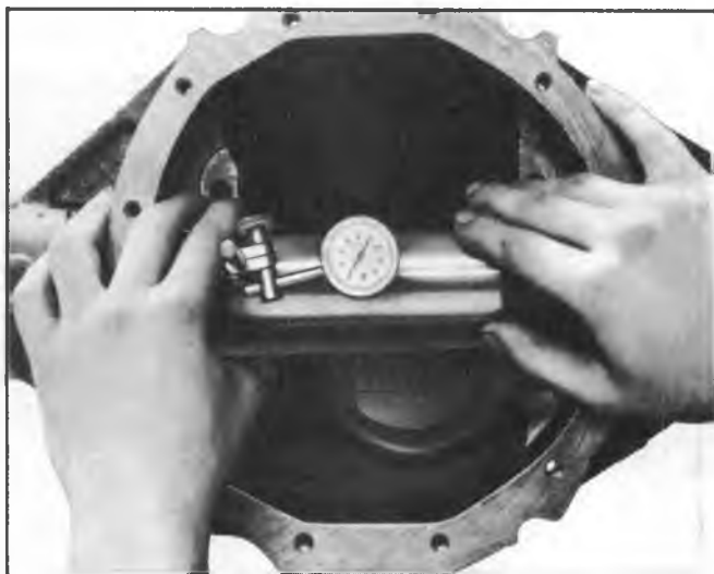
Fig. 14B—Measuring Drive Pinion Shim Requirement
