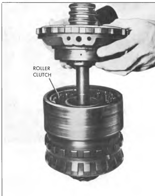
Fig. 39T--Removing Center Support Assembly
