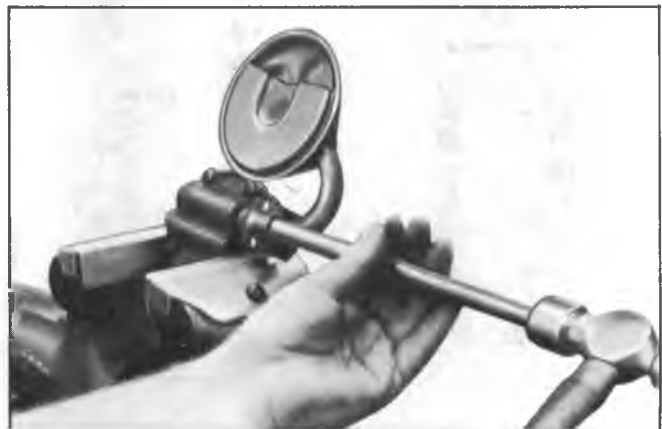
Fig. 38--Installing Screen ("Small V8")
