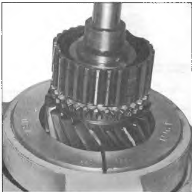
Fig. 9X—Removing 3-4 Synchronizer and Third Speed Gear
