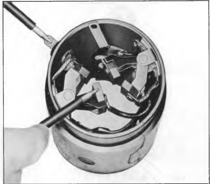
Fig. 6S--Field Coil Open Circuit Test
