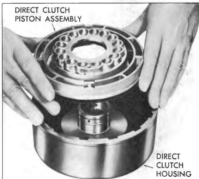
Fig. 83T--Removing Direct Clutch Piston Assembly
