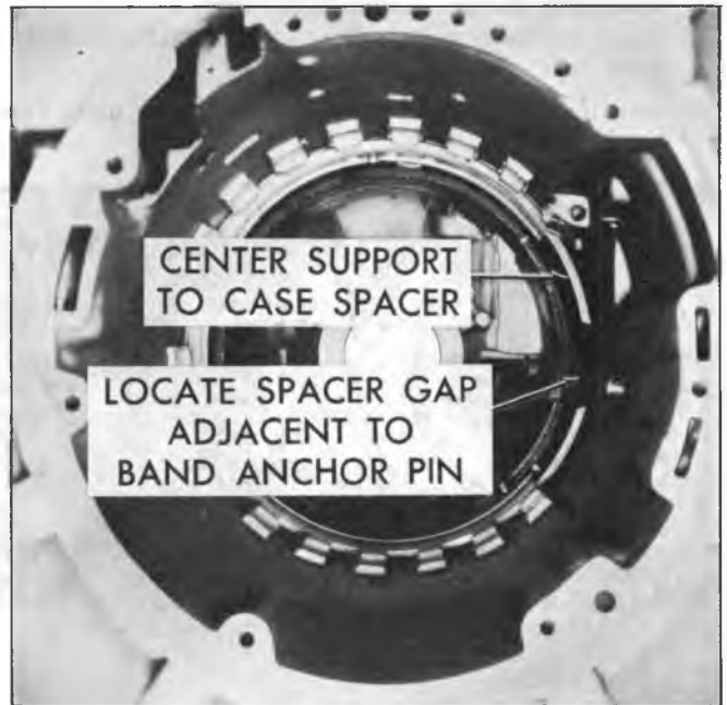
Fig. 129T-A--Installing Center Support to Case Spacer
