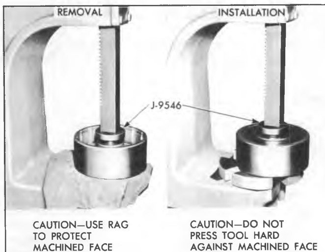
Fig. 21PG—Removing and Installing Clutch Drum Bushing
