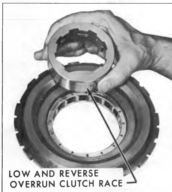
Fig. 92M--Removing Overrun Clutch Inner Race
