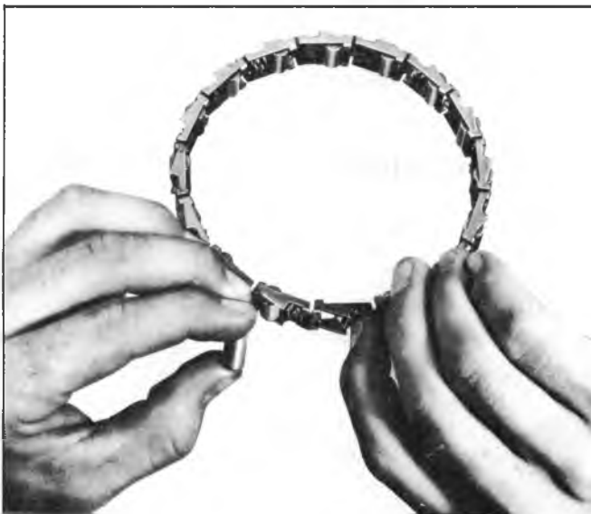
Fig. 123T--Installing Roller into Roller Clutch Cage
