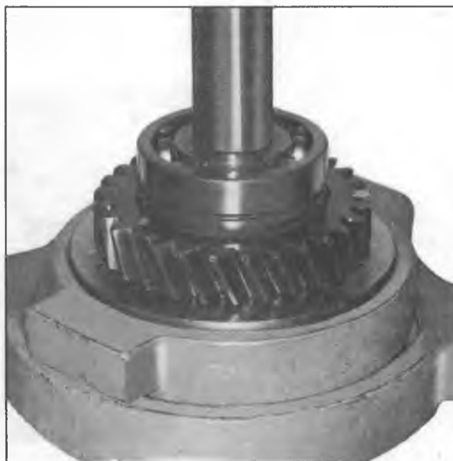
Fig. 11X—Removing Rear Bearing and First Speed Gear
