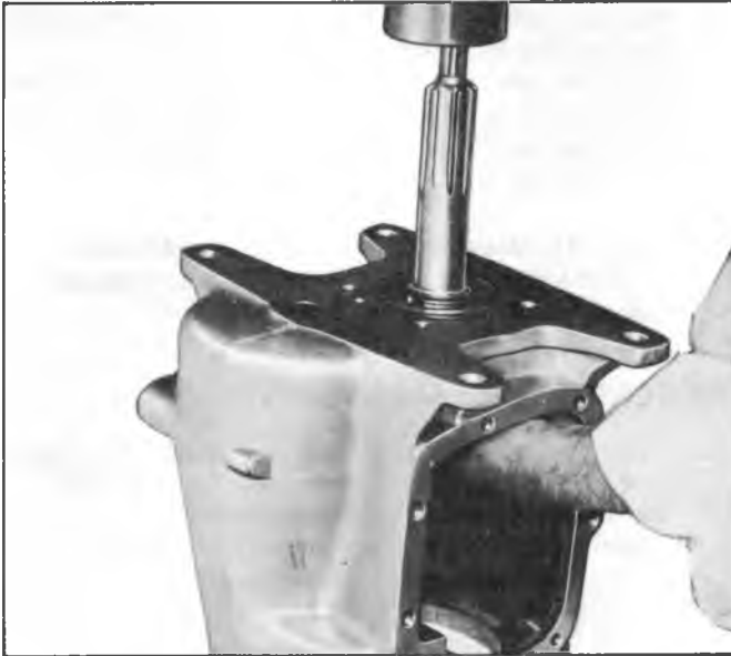
Fig. 7B—Removing Main Drive Gear
