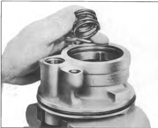
Fig. 28--Installing Pressure Plate Spring
