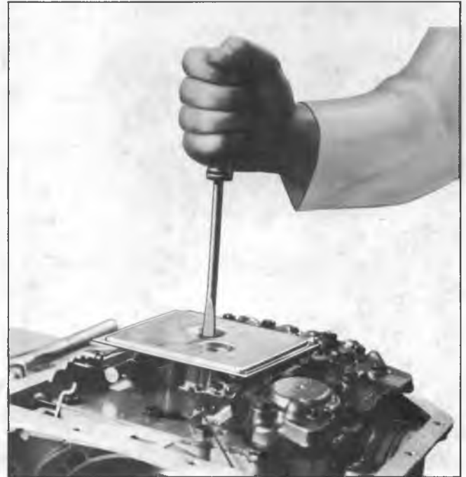
Fig. 11M--Removing Oil Pump Suction Screen (Strainer) from Valve Body
