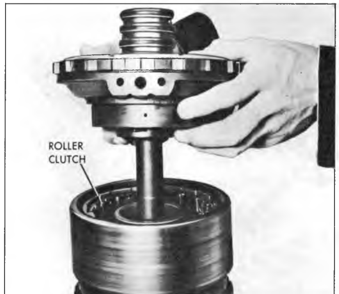
Fig. 125T--Installing Center Support to Reaction Carrier
