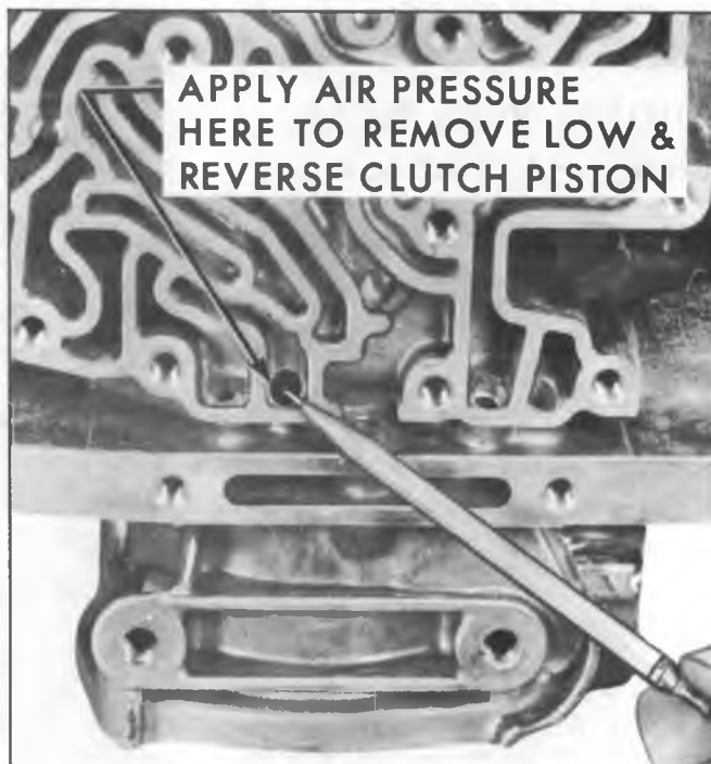
Fig. 48M--Removing Low and Reverse Clutch Piston
