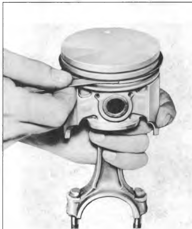
Fig. 59—Measuring Ring Groove Clearance
