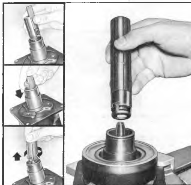
Fig. 13—Replacing Seal and "O" Ring
