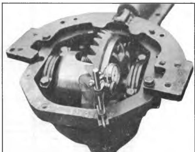
Fig. 26C--Checking Ring Gear Runout
