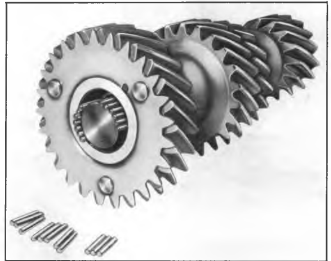
Fig. 15B—Loading Countergear Bearings Using J-22246
