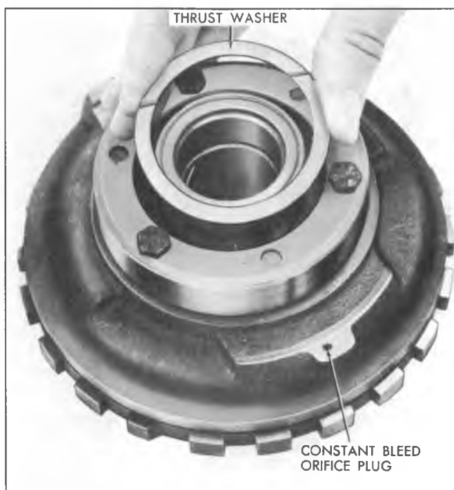
Fig. 40T--Removing Center Support Thrust Washer
