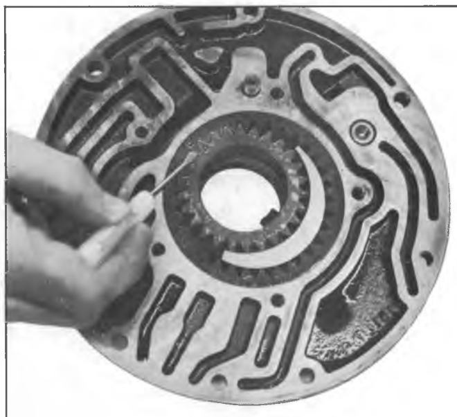
Fig. 65M--Installing Pump Drive and Driven Gears
