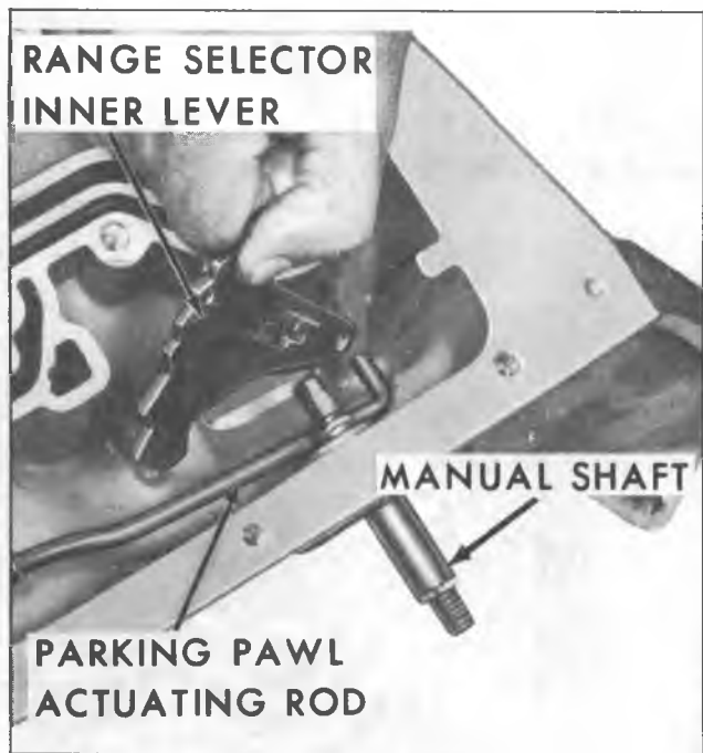
Fig. 21M—Removing Manual Shaft and Inner Lever and Parking Pawl Actuator Rod from Case
