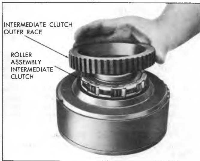
Fig. 92TA-Installing Intermediate Clutch Outer Race to Direct Clutch
