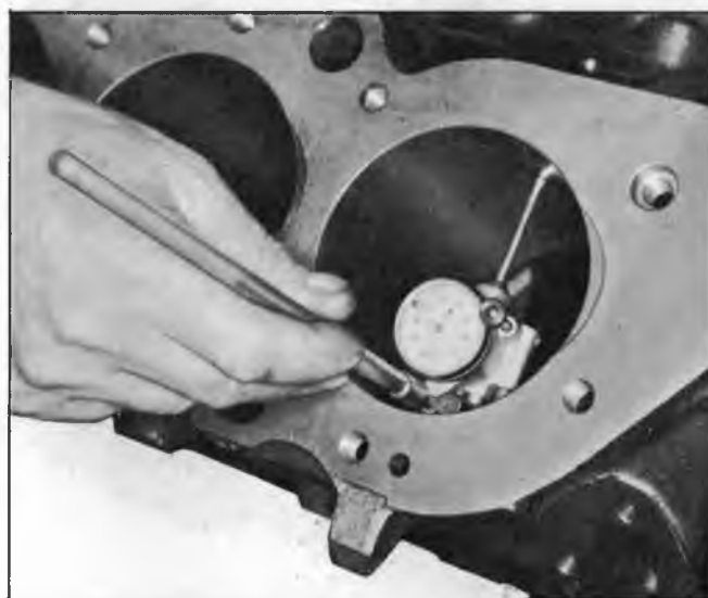
Fig. 70—Measuring Cylinder Bore
