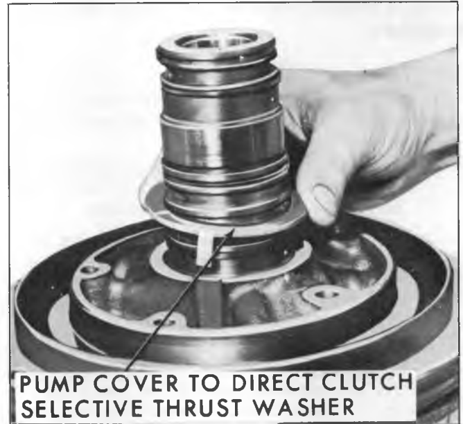
Fig. 107M--Pump Cover to Direct Clutch Selective Thrust Washer
