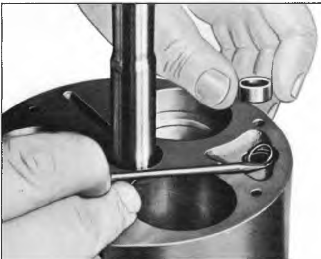
Fig. 26—Installing Discharge Crossover Tube Front "O" Ring and Spacer
