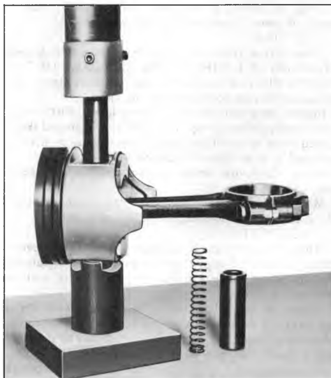
Fig. 51--Removing Piston Pin (In-Line and "Small V8")
