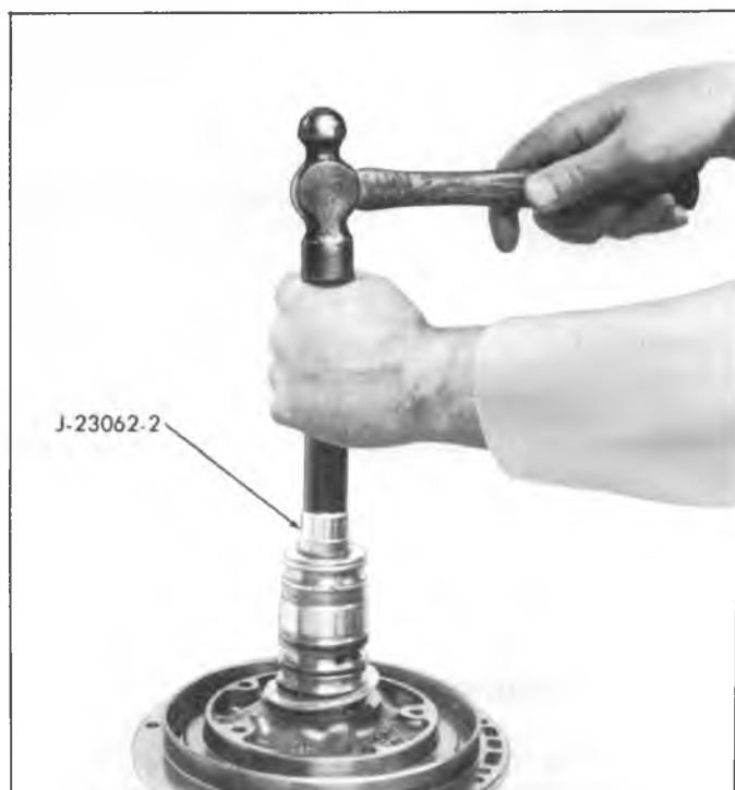
Fig. 100M--Installing Rear and Center Stator Shaft Bushings
