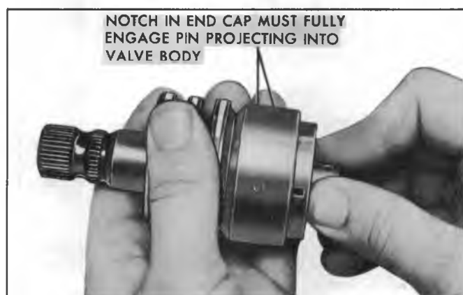
Fig. 46--Installing Stub Shaft Assembly
