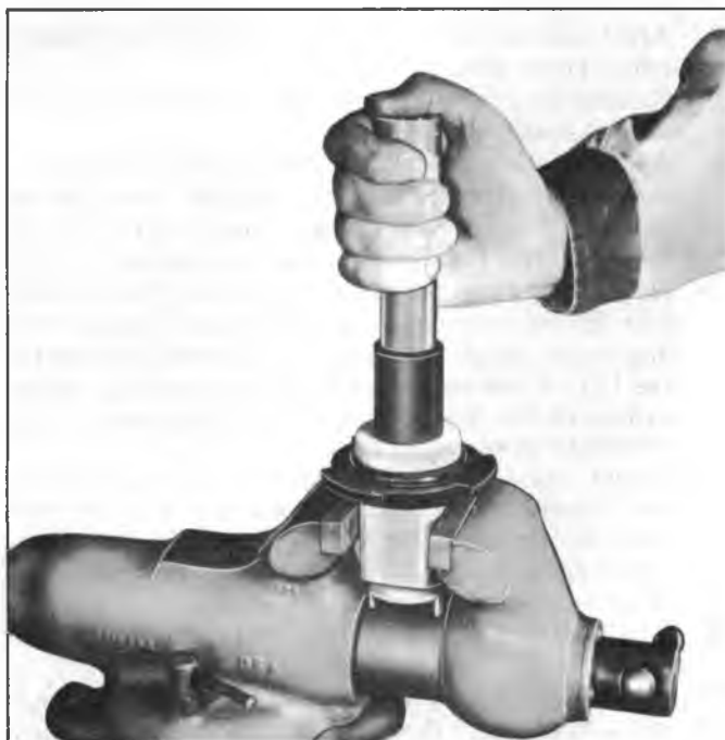
Fig. 12H--Seating Floating Control Valve Assembly with Installer J-23175
