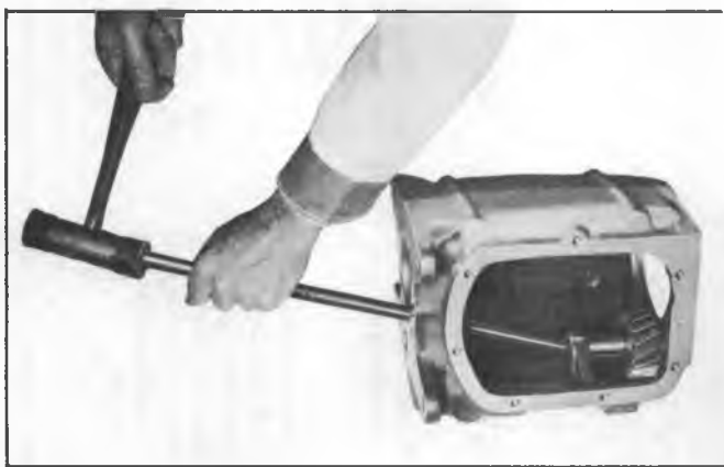
Fig. 3A—Removing Reverse Idler Shaft
