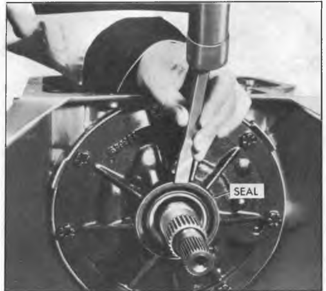
Fig. 20T--Removing Front Seal
