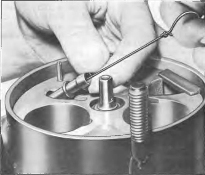
Fig. 16—Removing Oil Inlet Tube and "O" Ring
