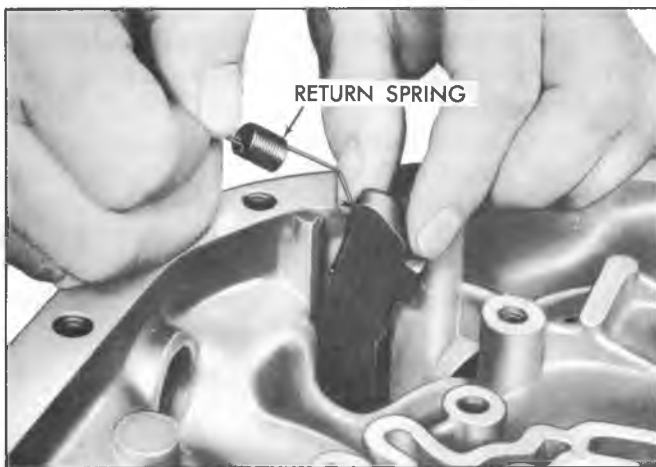
Fig. 27T--Removing Parking Pawl Return Spring
