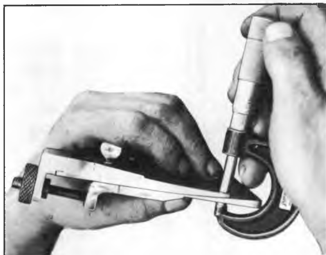
Fig. 23C--Measuring Gauge Plate Thickness
