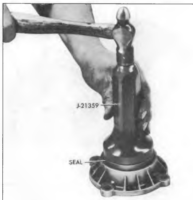
Fig. 19C—Installing Rear Bearing Retainer Seal
