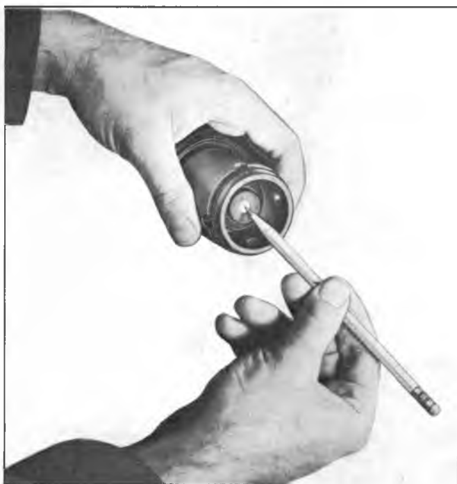
Fig. 7H--Removing Reaction Piston and Reaction Disc From Secondary Power Piston
