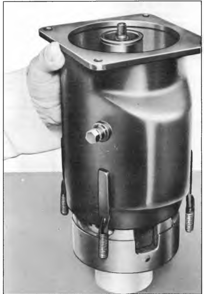
Fig. 27—Installing Shell Over Internal Mechanism
