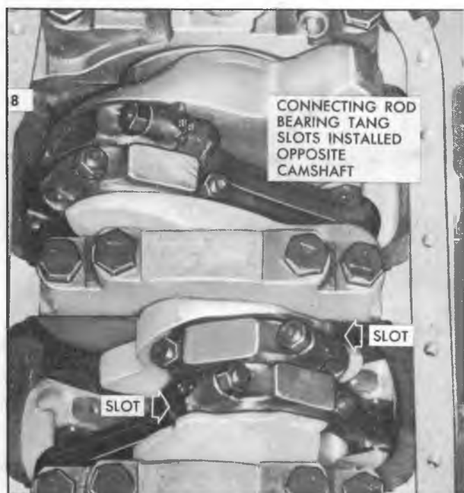
Fig. 60-Connecting Rods-Installed Position V8
