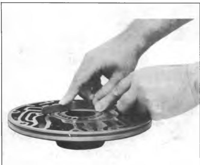
Fig. 64M--Checking Pump Body to Gear Face Clearance
