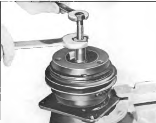
Fig. 3—Removing Hub and Drive Plate Assembly
