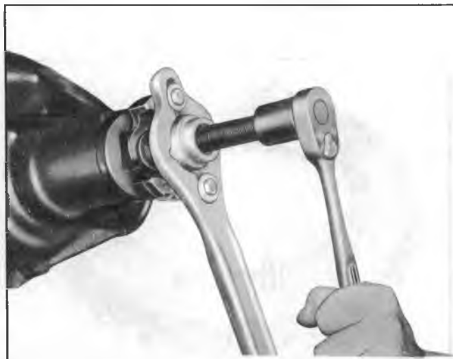
Fig. 6B-Drive Pinion Flange Removal
