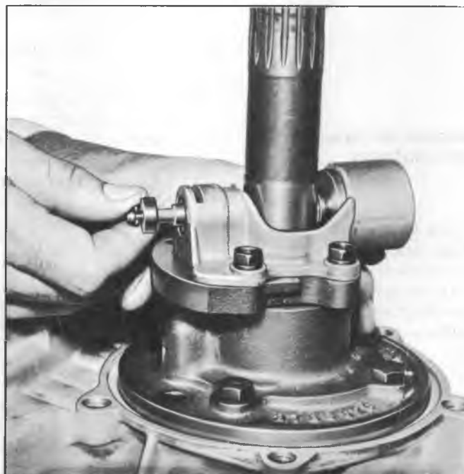
Fig. 4PG--Removing Governor Valve and Shaft
