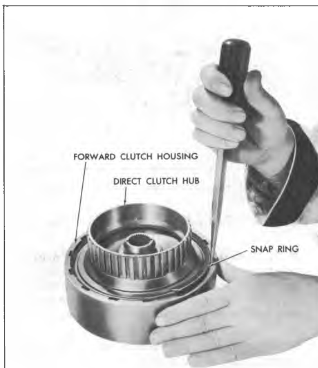
Fig. 67T--Removing Forward Clutch Housing to Direct Clutch Hub Snap Ring
