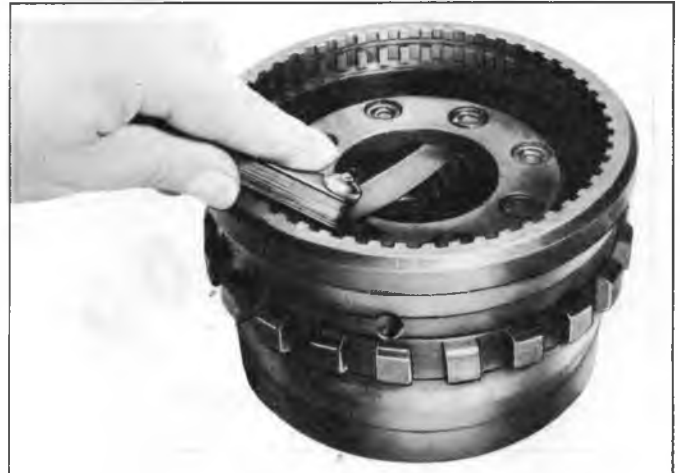
Fig. 106T--Checking Output Carrier Pinion End Play
