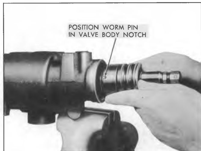
Fig. 55--Valve to Worm Alignment
