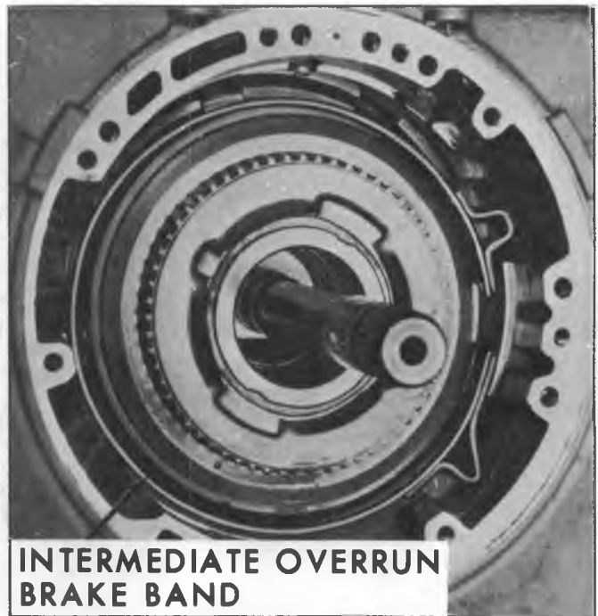
Fig. 32M--Removing Intermediate Overrun Brake Band
