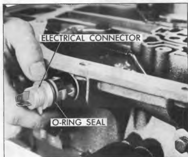
Fig. 15T--Removing Electrical Connector and "O" Ring Seal
