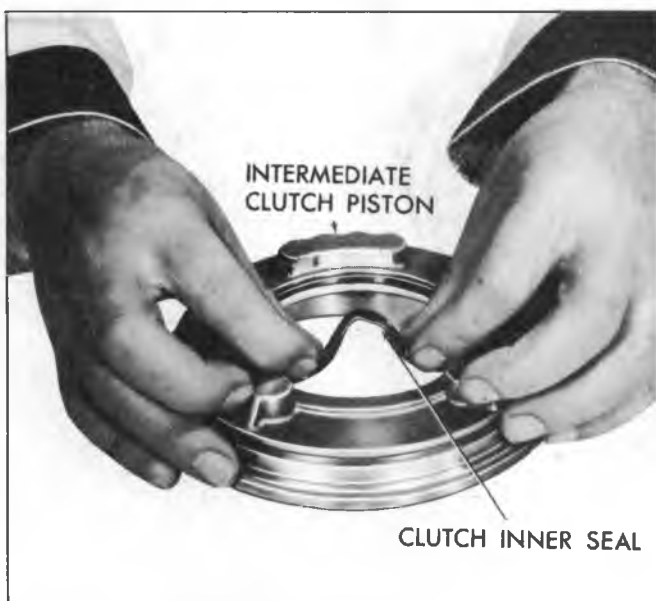
Fig. 100T—Installing Intermediate Clutch Inner Seal
