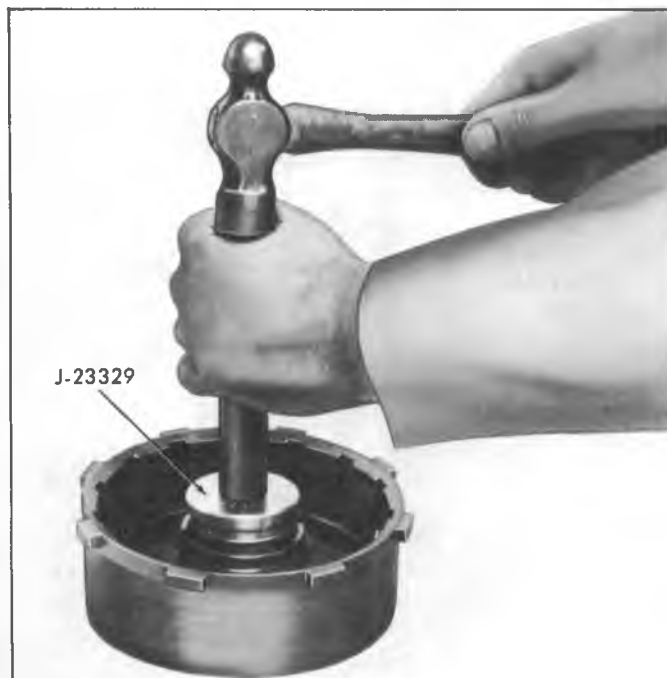
Fig. 105M--Installing Direct Clutch Drum Bushing
