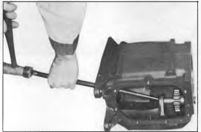
Fig. 7X--Removing Reverse Idler Gear Shaft
