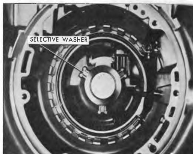
Fig. 37T--Removing Selective Washer
