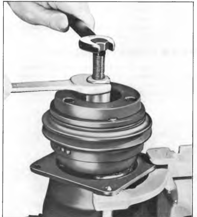
Fig. 5—Installing Hub and Drive Plate Assembly
