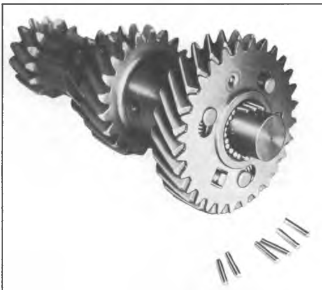
Fig. 6A-Loading Counter gear Bearings w/Tool J-22246
