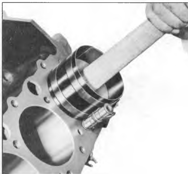
Fig. 62-Installing Connecting Rod and Piston Assemblies
