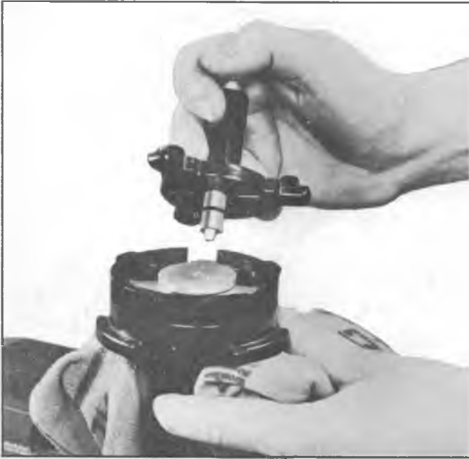
Fig. 9A—Installing Reaction Retainer on Power Piston
