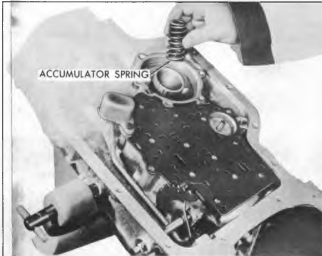
Fig. 147T--Installing Rear Accumulator Spring
