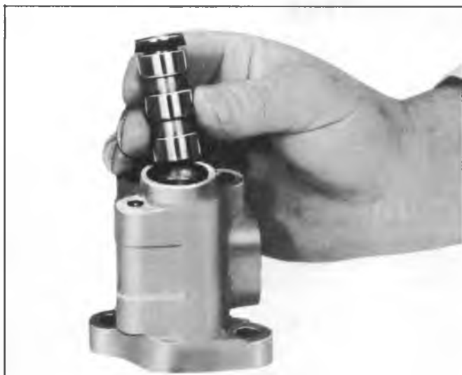
Fig. 65--Removing Spool from Housing
