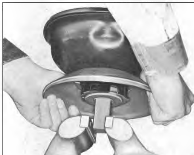
Fig. 4A-Separating Power Piston from Support Plate
