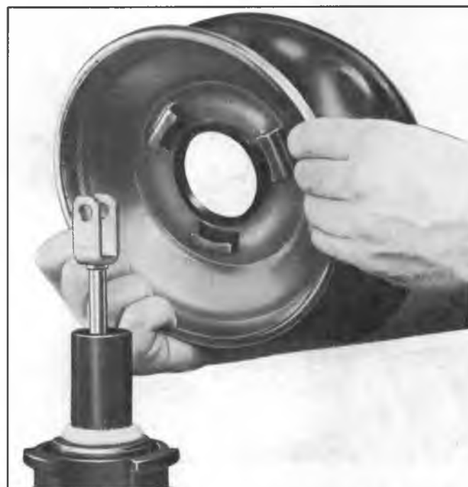
Fig. 8A—Installing Power Piston to Support Plate
