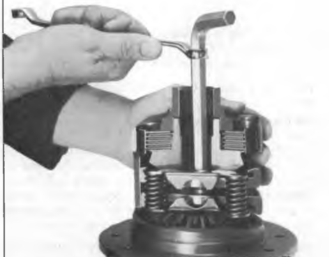
Fig. 6E-- C-Clamp and Bar Stock Installed for Spring Removal
