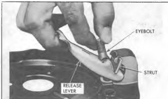
Fig. 5E-Removing Levers (Step 2)
