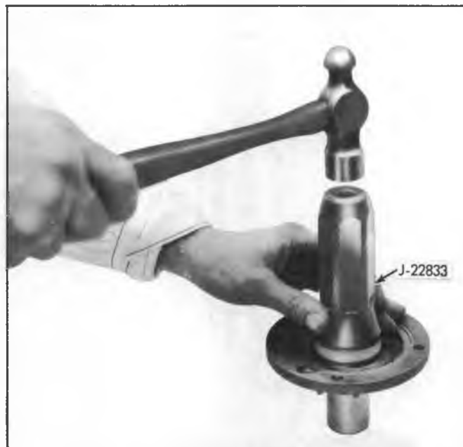
Fig. 13Q--Installing Bearing Retainer Oil Seal
