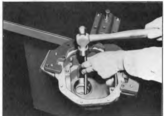
Fig. 10C--Removing Pinion Bearing Cup
