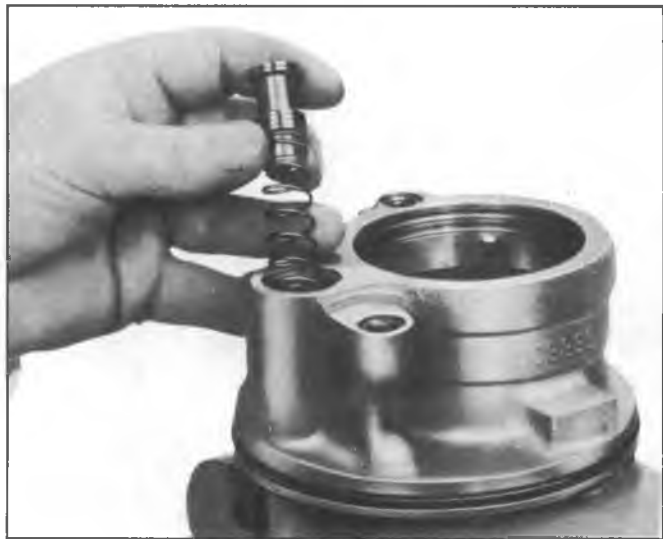
Fig. 30--Installing Flow Control Valve
