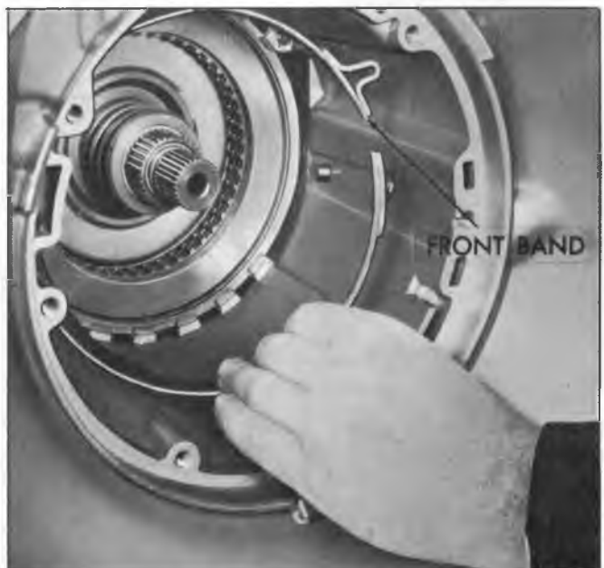
Fig. 30T--Removing Front Band
