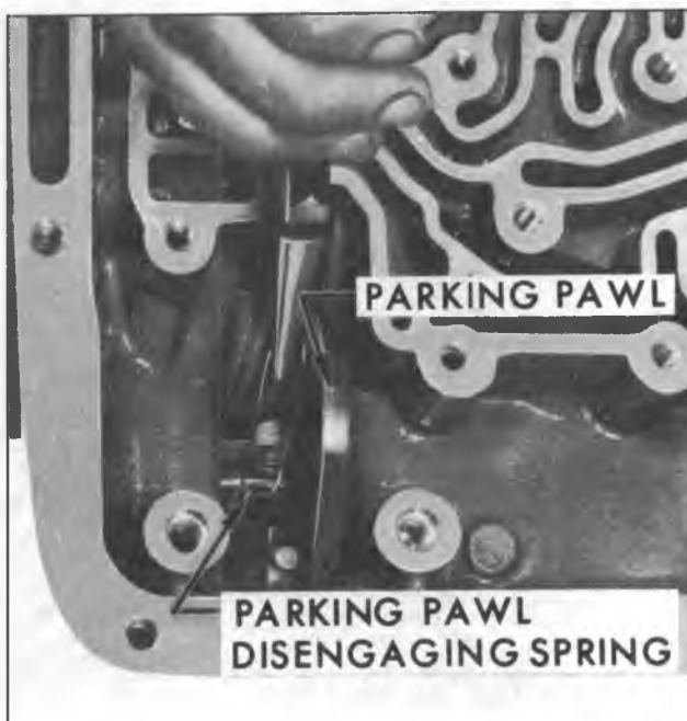
Fig. 24M—Removing Parking Pawl Disengaging Spring
