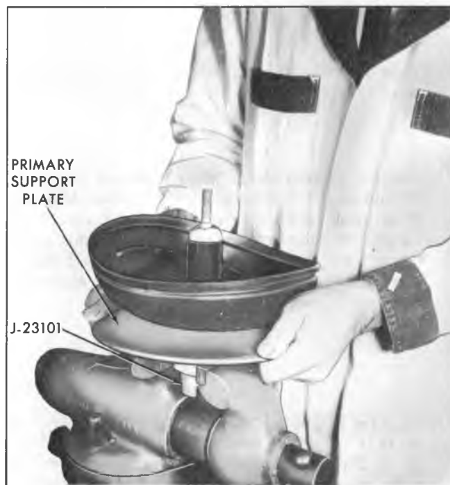
Fig. 9H--Locking or Unlocking Primary Support Plate From Primary Power Piston
