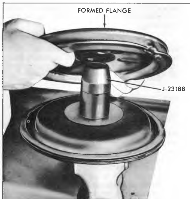
Fig. 14H--Positioning Housing Divider Over Secondary Bearing Protector Tool J-23188
