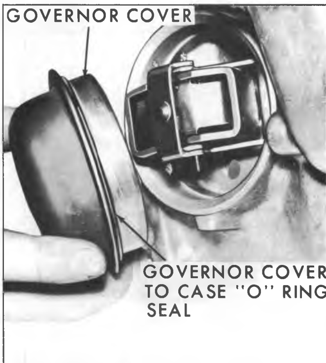
Fig. 8M--Governor Cover and "O" Ring Seal
