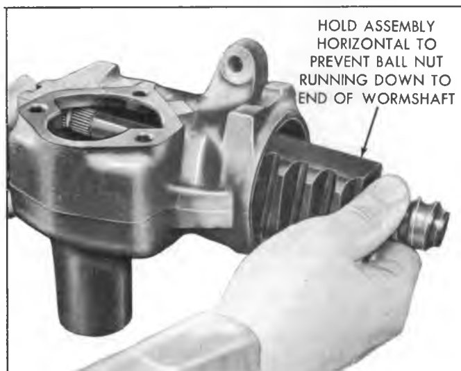
Fig. 6—Removing the Wormshaft and Ball Nut—Typical
