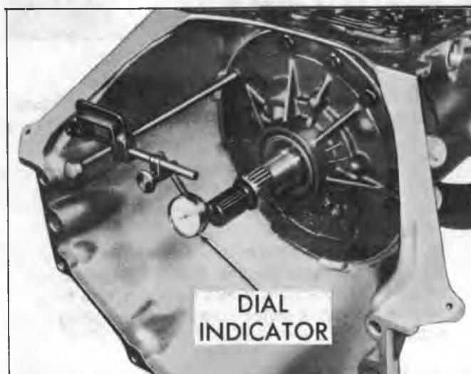
Fig. 139T--Checking Front Unit End Play
