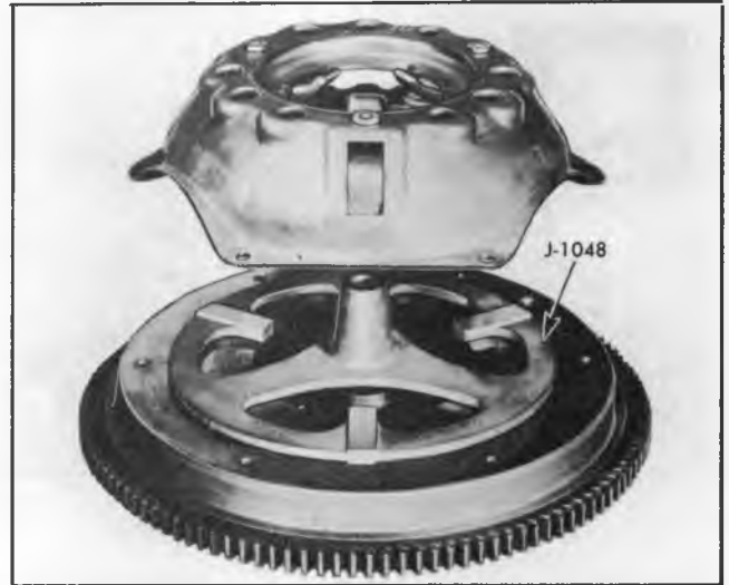
Fig. 11E—Gauge Plate Position
