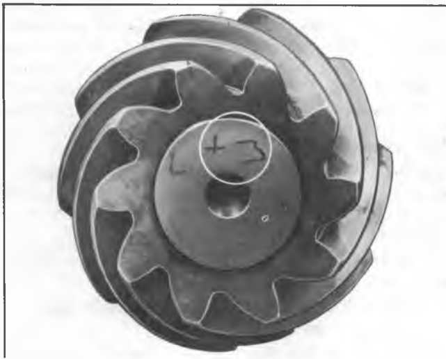
Fig. 7D-Marking From Nominal on Pinion
