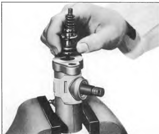
Fig. 66--Removing Valve Parts from Shaft
