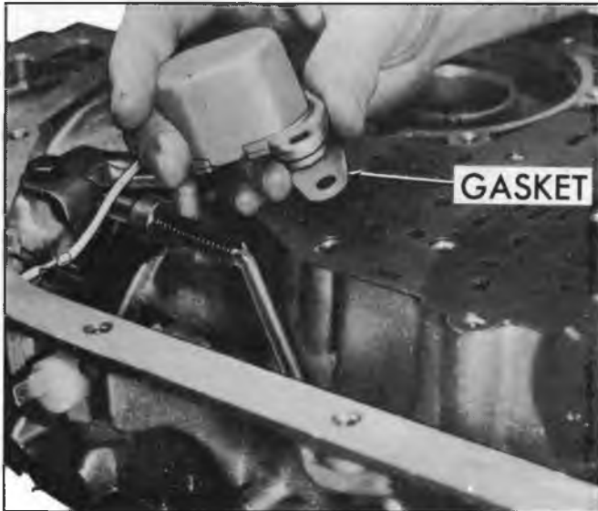
Fig. 144T--Installing Detent Solenoid and Gasket
