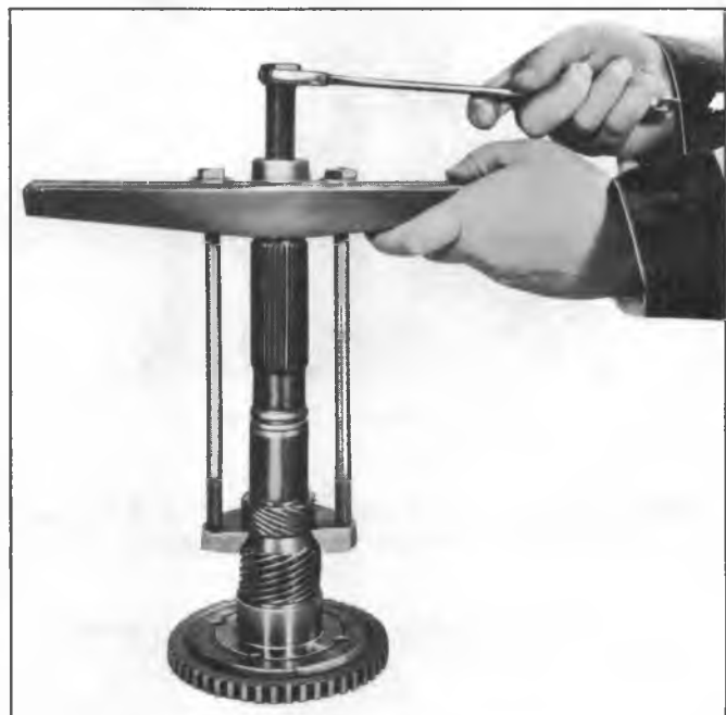
Fig. 47T-A--Removing Steel Speedometer Drive Gear
