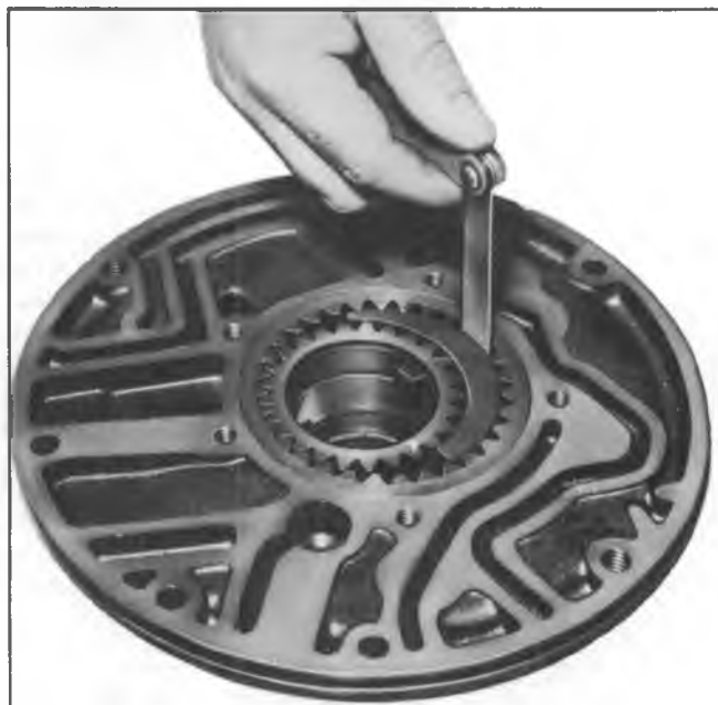
Fig. 18PG—Driven Gear to Crescent Clearance
