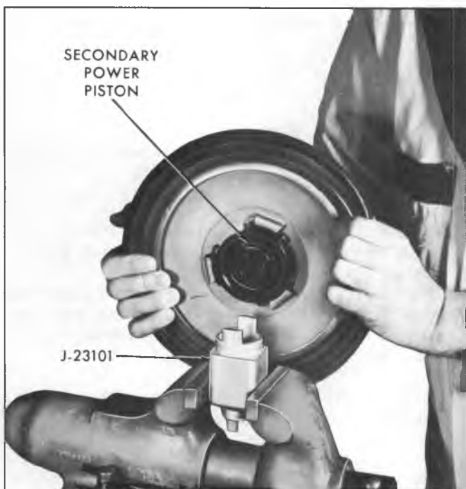
Fig. 4H—Positioning Secondary Power Piston in Tool J-23101 (Large Dia. End Up)
