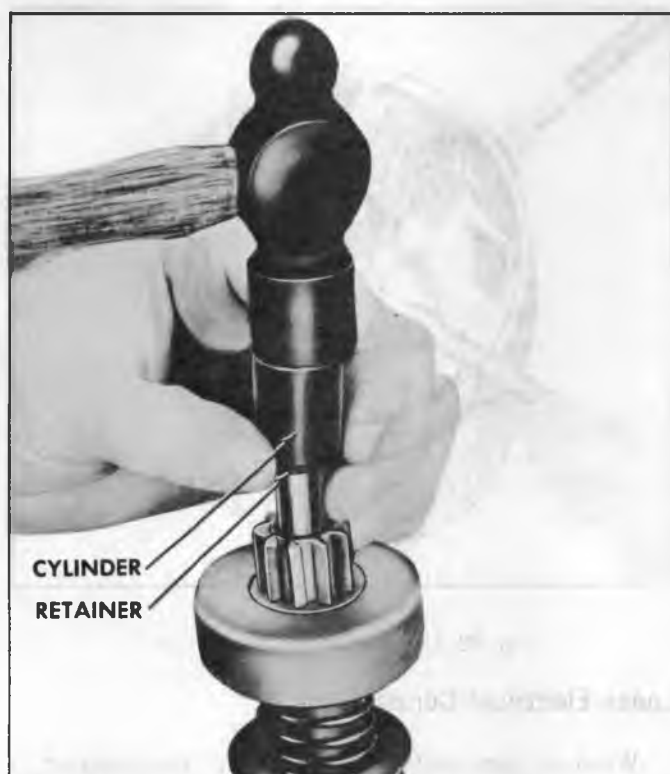
Fig. 3S--Driving Retainer Off Snap Ring
