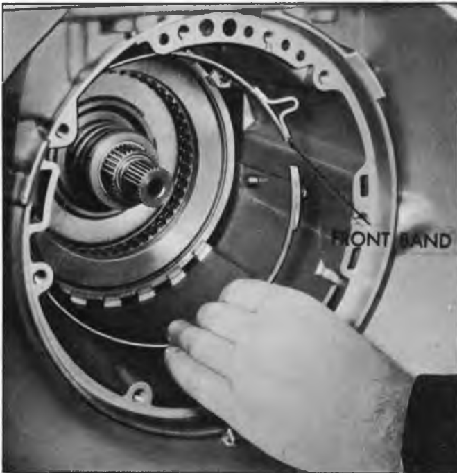
Fig. 133T--Installing Front Band
