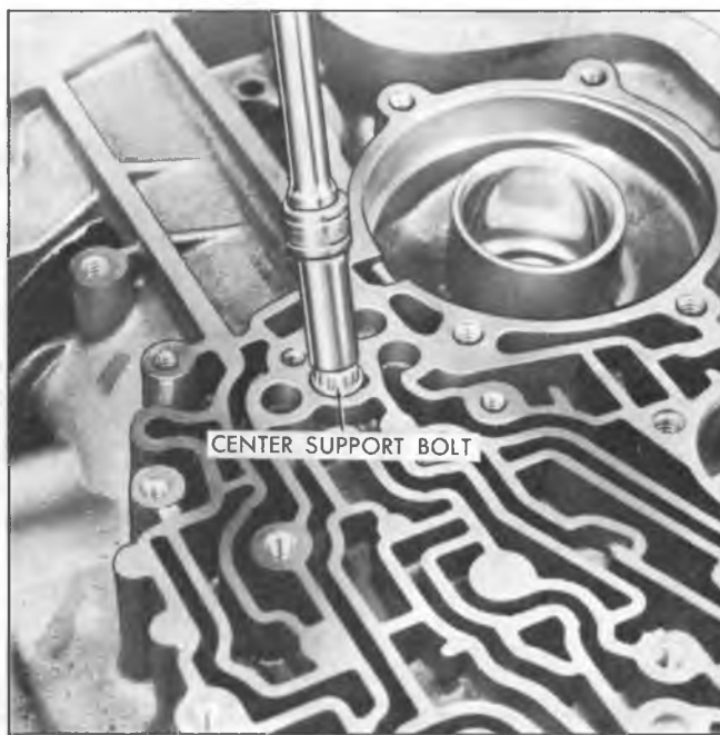
Fig. 33T--Removing Center Support Bolt
