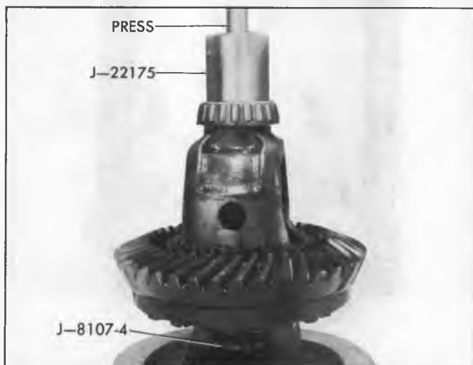
Fig. 3A-Differential Bearing Installation (P-Type Axle)
