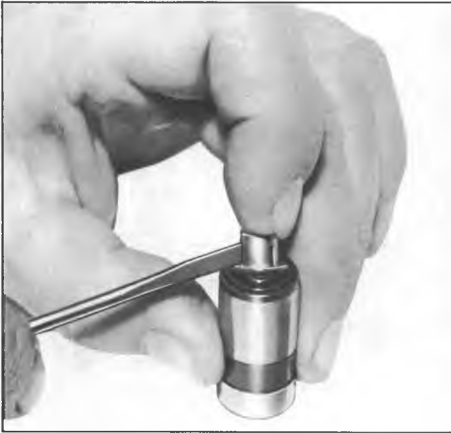
Fig. 31—Removing Ball Check Valve
