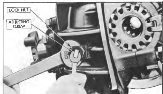
Fig. 15F--Ring Gear Thrust Pad Adjustment
