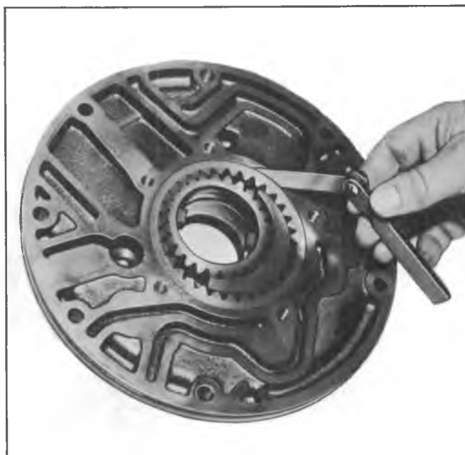
Fig. 17PG—Checking Driven Gear to Pump Body Clearance
