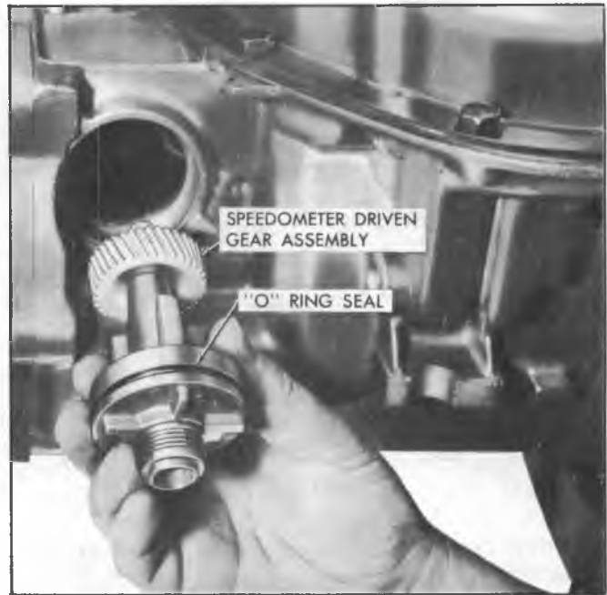
Fig. 155T—Installing Speedometer Driven Gear and Sleeve
