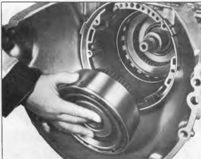
Fig. 23T--Removing Direct Clutch Assembly
