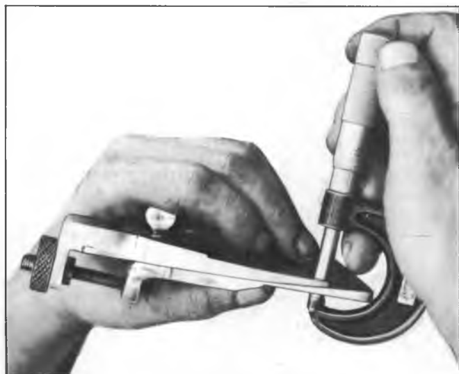
Fig. 21A—Measuring Gauge Thickness
