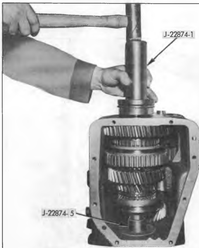
Fig. 23Q—Installing Mainshaft Rear Bearing
