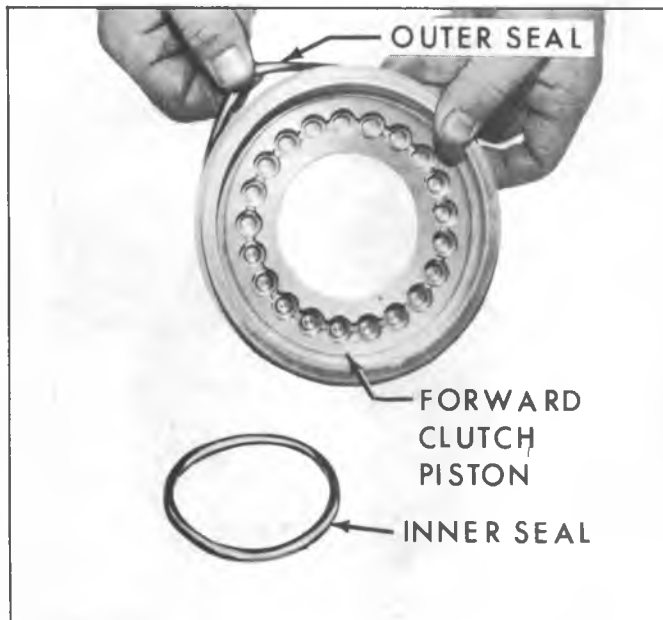
Fig. 83M--Removing Forward Clutch Piston Inner and Outer Seals
