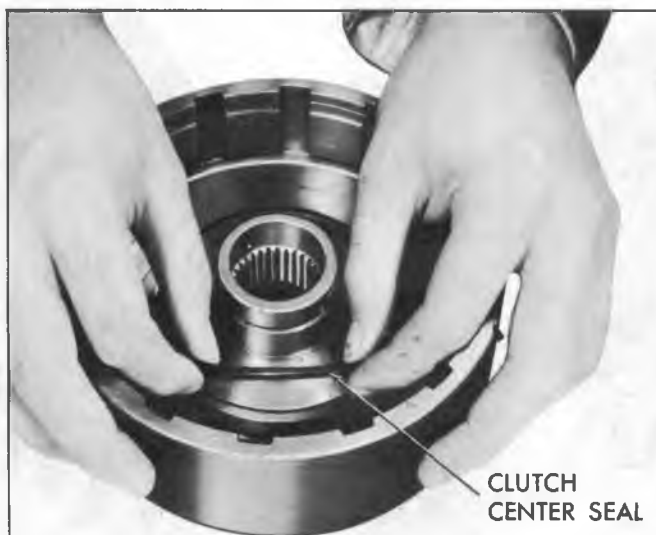
Fig. 87T—Installing Direct Clutch Center Seal
