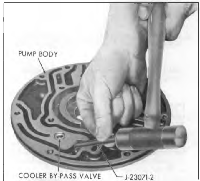
Fig. 62M--Removing Cooler By-Pass Valve Seat
