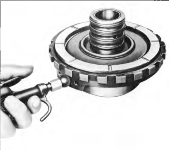
Fig. 104T--Air Checking Intermediate Clutch Piston
