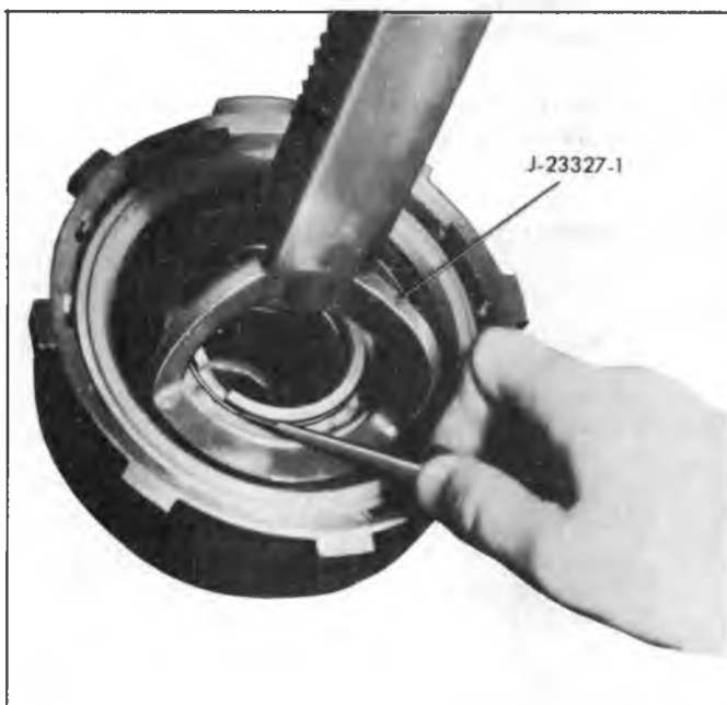
Fig. 74M--Compressing Direct Clutch Spring Seat
