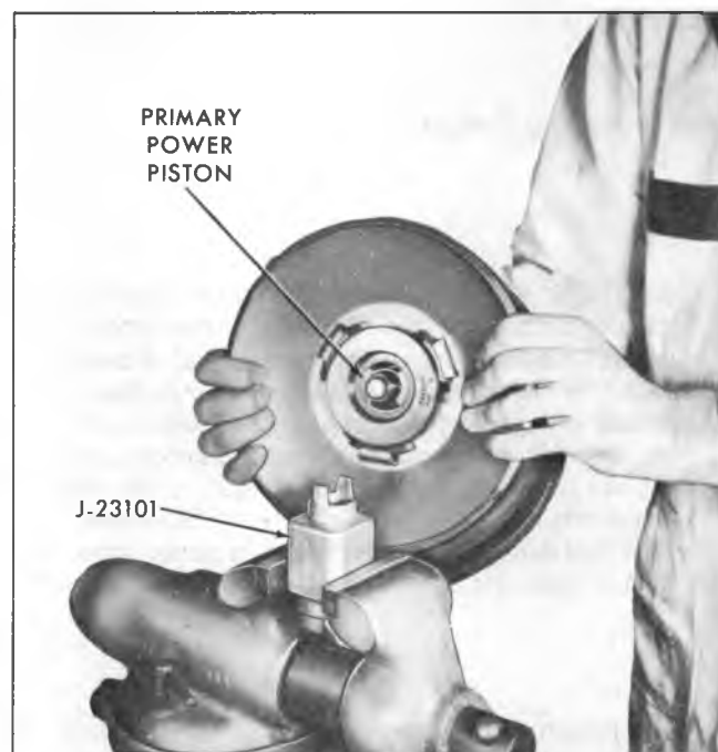
Fig. 8H--Positioning Primary Power Piston in Tool J-23101 (Small Dia. End Up)
