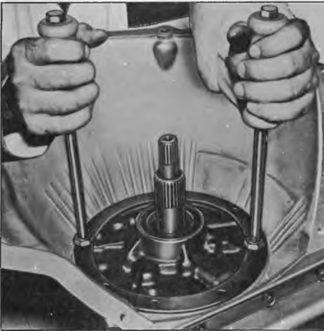
Fig. 6PG-Removing Oil Pump
