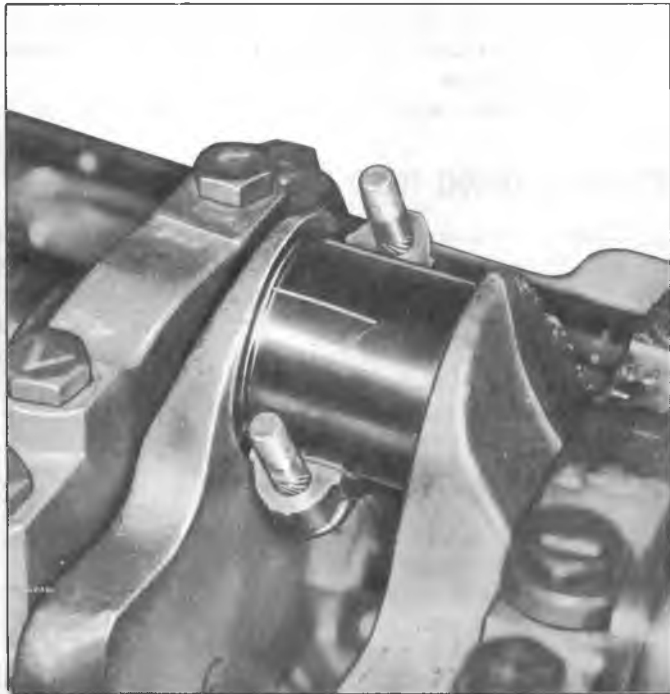
Fig. 44--Gauging Plastic on Crankpin
