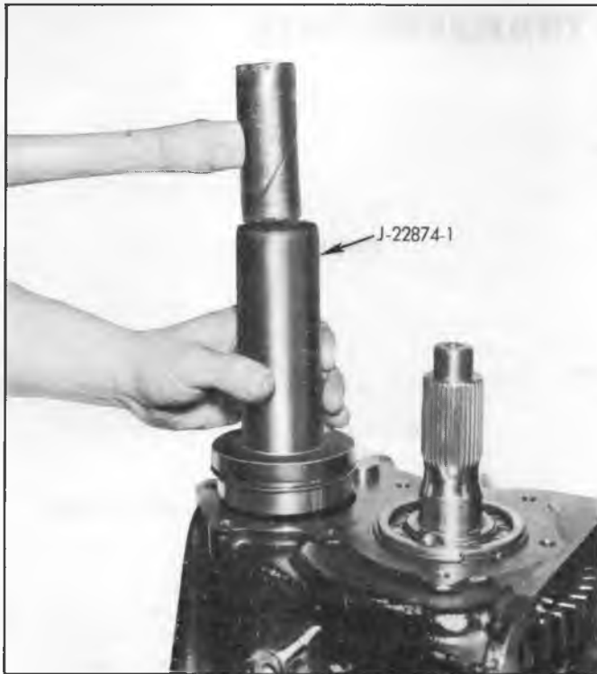
Fig. 25Q--Installing Countergear Rear Bearing
