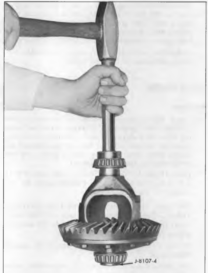
Fig. 4A-Differential Bearing Installation (Except P-Type Axles)
