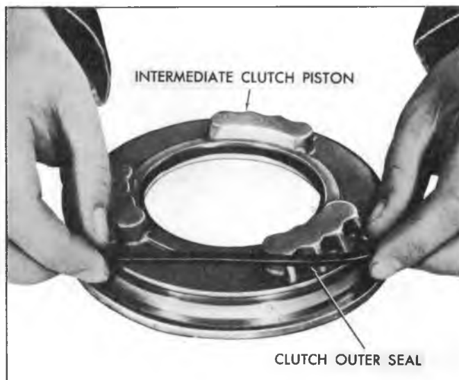
Fig. 101T—Installing Intermediate Clutch Outer Seal
