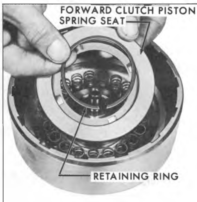
Fig. 78M--Installing Direct Clutch Springs, Spring Seat and Retaining Ring
