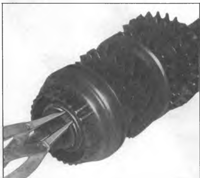
Fig. 10X—Rear Bearing to Mainshaft Snap Ring
