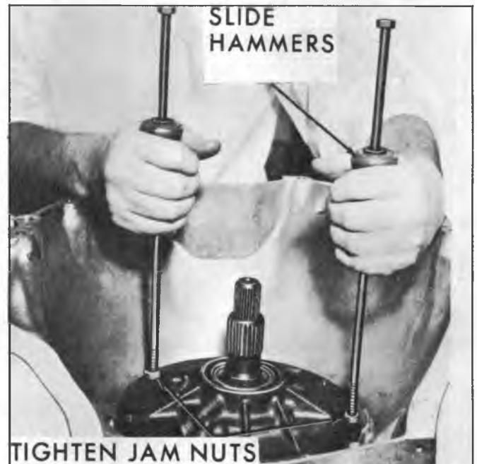
Fig. 28M--Removing Pump from Case
