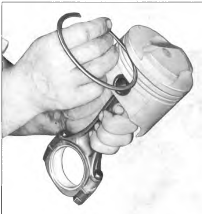
Fig. 57—Checking Ring In Groove
