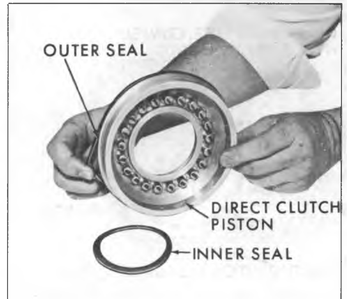
Fig. 75M--Removing Direct Clutch Outer and Inner Seals
