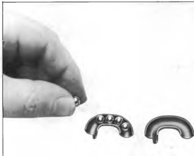
Fig. 13—Filling Ball Guides—Corvette
