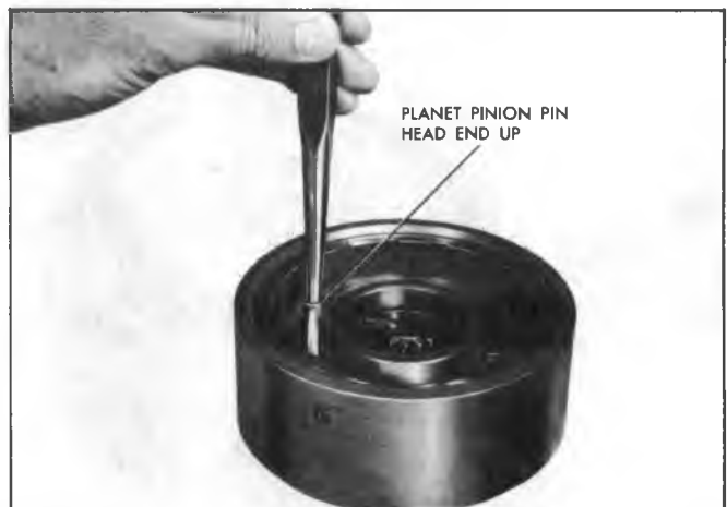
Fig. 109T-Installing Planet Pinion Pin
