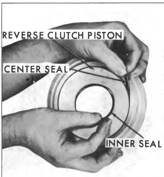
Fig. 50M—Removing Low and Reverse Clutch Piston Center and Inner Seal
