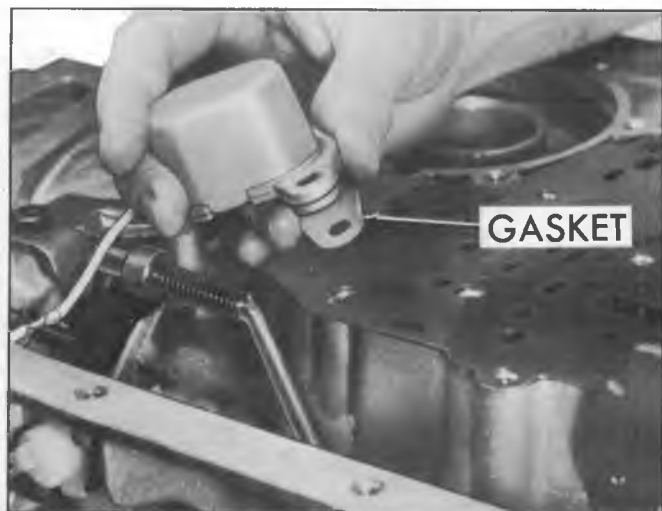
Fig. 14T--Removing Detent Solenoid and Gasket
