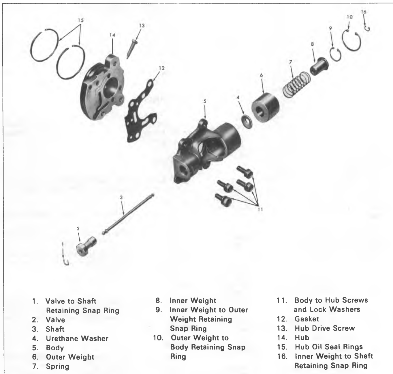
Fig. 26PG-Governor-Exploded View
