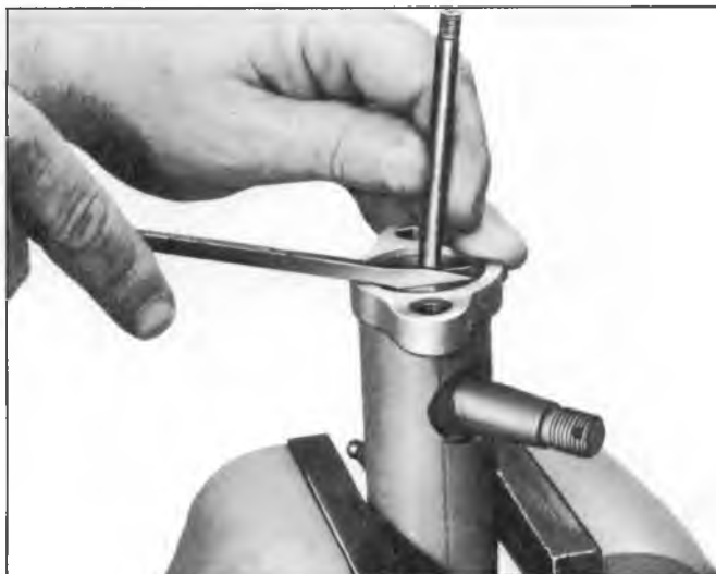
Fig. 69--Turning Adjuster Plug out of Sleeve
