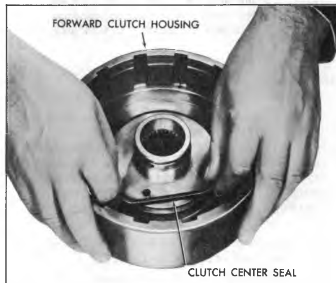
Fig. 72T--Removing Forward Clutch Center Seal
