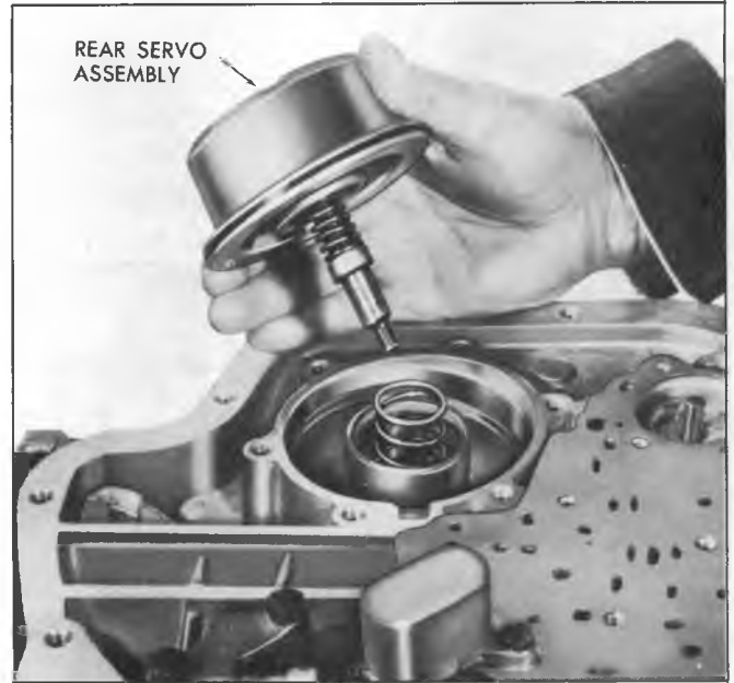
Fig. 12T-Removing Rear Servo Assembly
