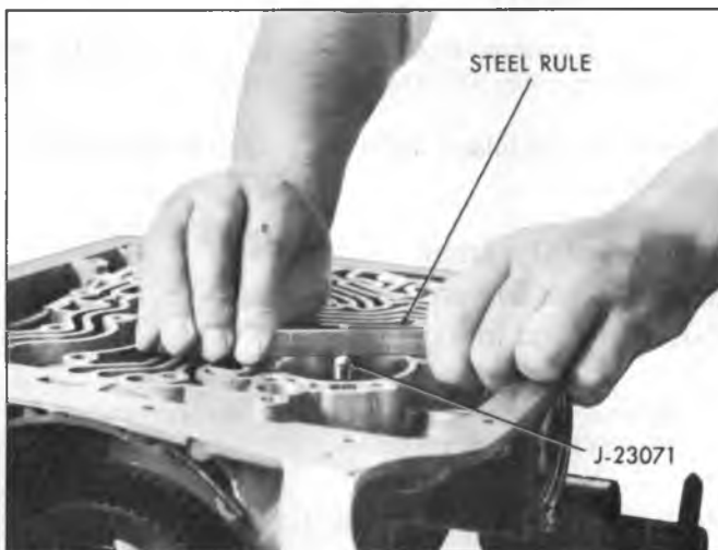
Fig. 111M—Gauging for Proper Apply Pin Selection
