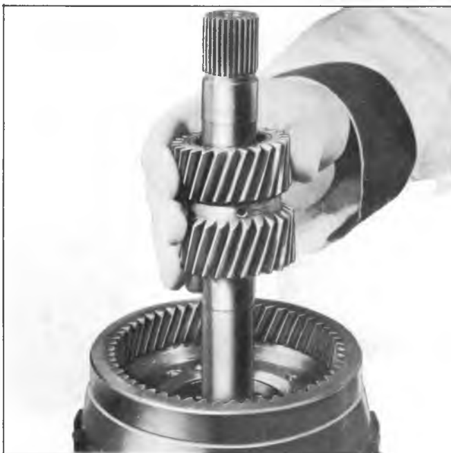
Fig. 42T--Removing Sun Gear
