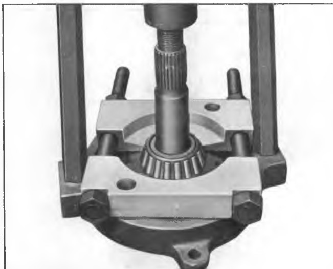
Fig. 8A—Removing Drive Pinion Rear Bearing.
