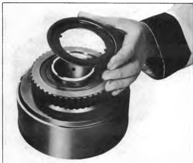
Fig. 94T-Installing Intermediate Clutch Retainer
