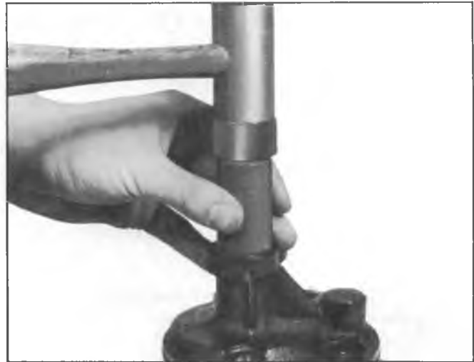
Fig. 21—Installing Seal Using Tool J-22670
