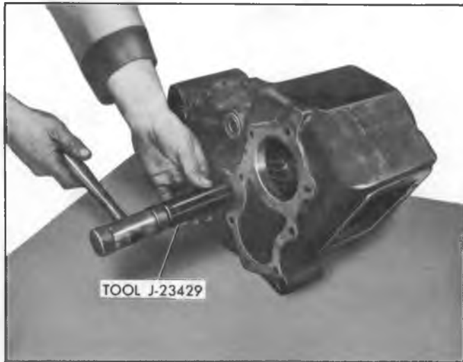
Fig. 8C--Removing Idler Gear Shaft
