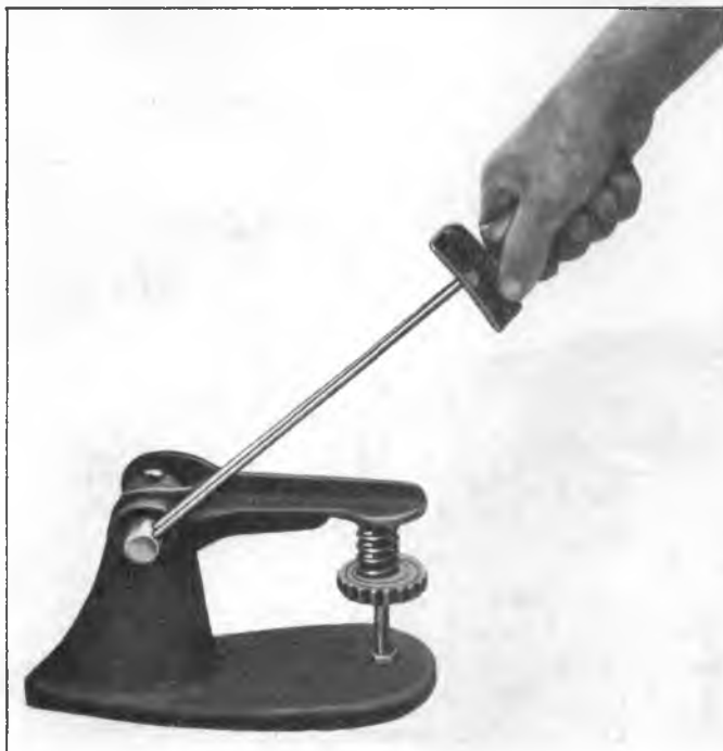
Fig. 17--Checking Valve Spring Tension
