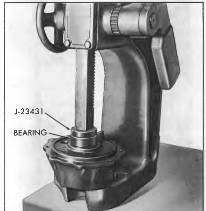
Fig. 17C--Installing Rear Output Shaft Housing Bearing
