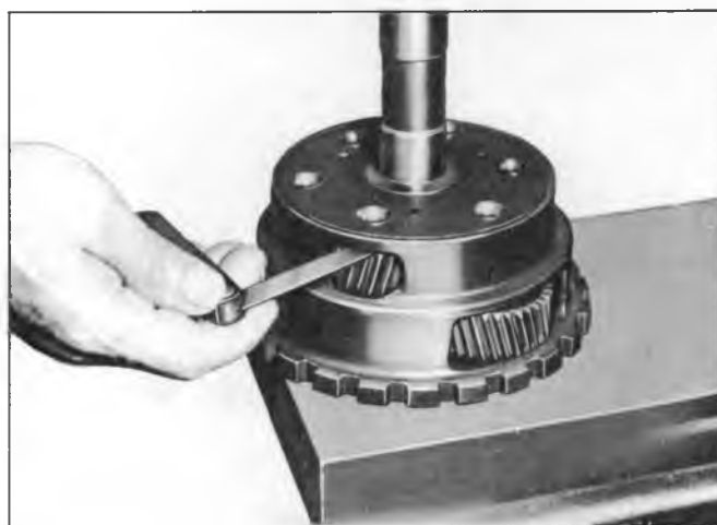
Fig. 23PG—Checking Planet Gear End Clearance
