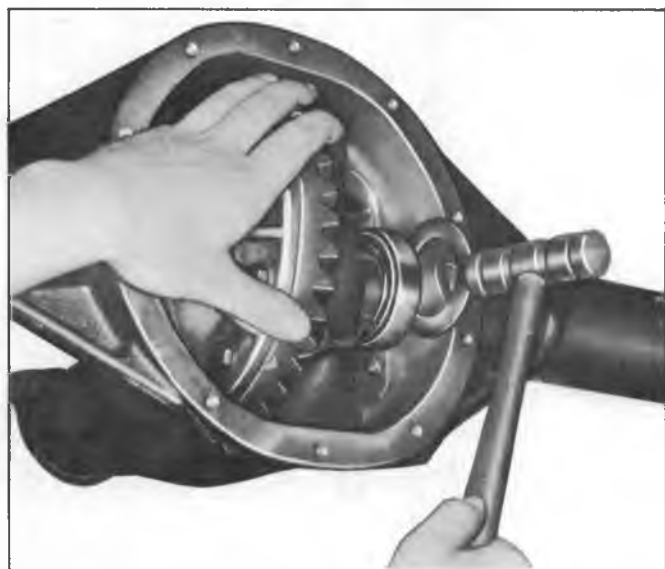
Fig. 22A—Installing Differential Shim
