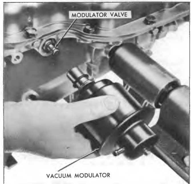
Fig. 153T--Installing Vacuum Modulator and Valve
