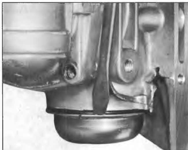
Fig. 7M--Removing Governor Cover
