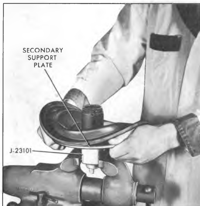
Fig. 6H--Locking or Unlocking Secondary Support Plate and Secondary Power Piston
