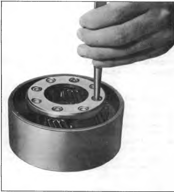
Fig. 107T-Removing Planet Pinion Pin
