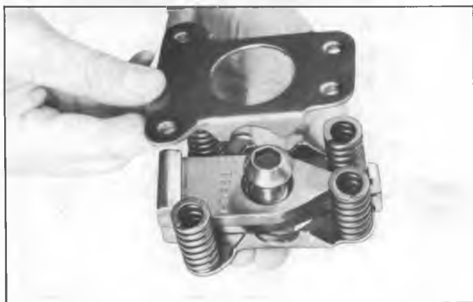
Fig. 13E—Installing Spring Pack Compression Tool (Corvette)
