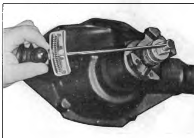
Fig. 18A-Measuring Drive Pinion Bearing Preload
