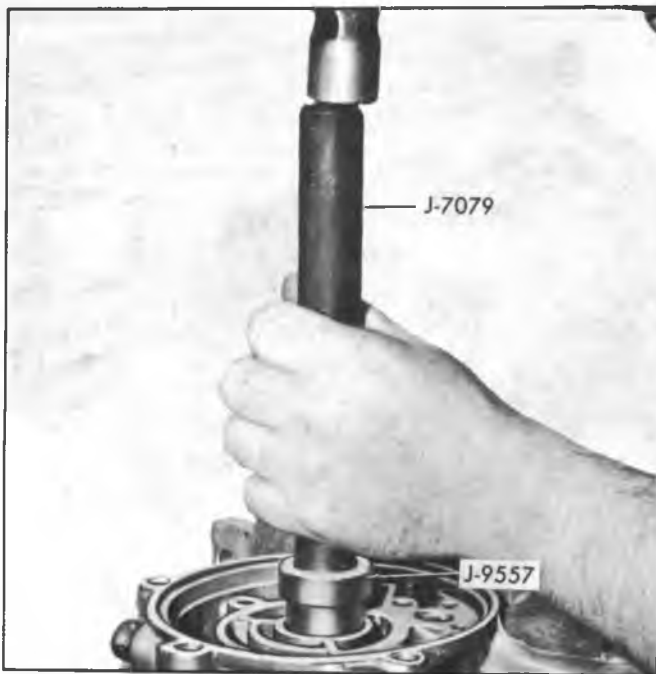
Fig. 28PG—Installing Case Rear Bushing
