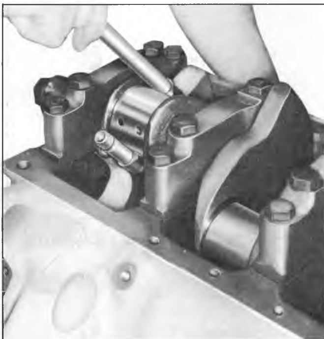
Fig. 48--Removing Connecting Rod and Piston Assemblies
