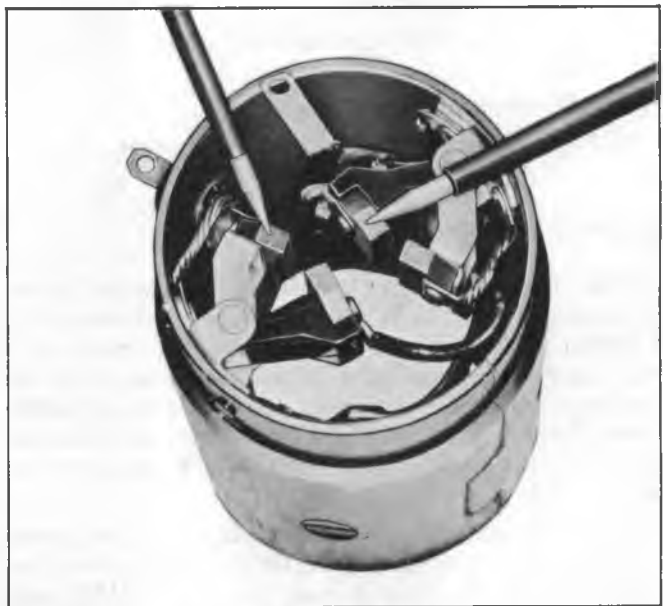
Fig. 7S--Field Coil Ground Test
