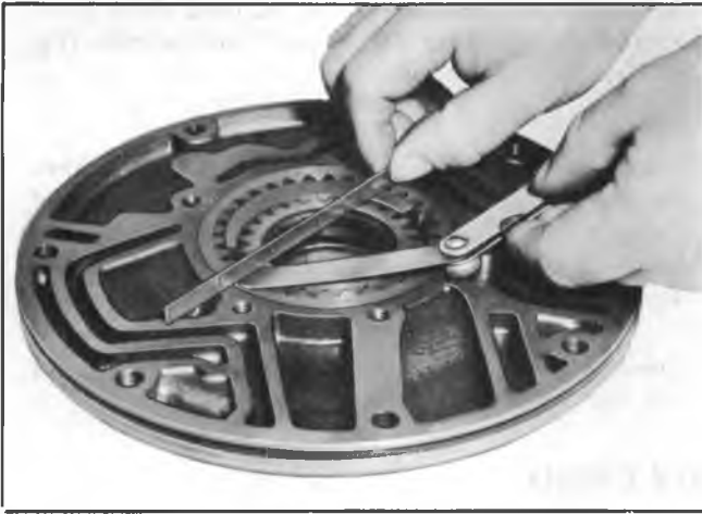
Fig. 19PG—Checking Gear End Clearance
