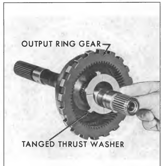
Fig. 44M--Removing Output Ring Gear Tanged Thrust Washer
