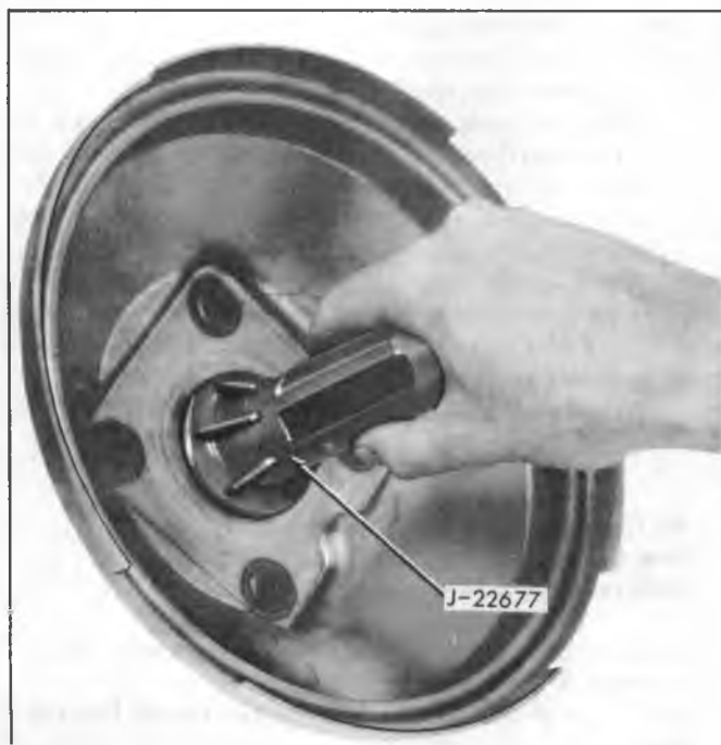
Fig. 7B—Installing Piston Bearing Seal
