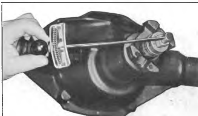
Fig. 20B—Measuring Drive Pinion Bearing Preload
