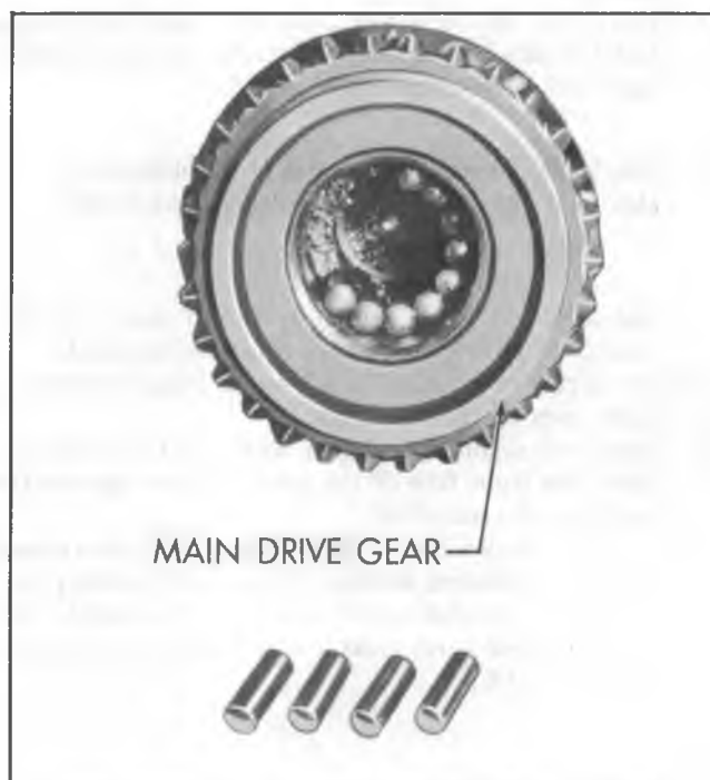
Fig. 24X—Loading Mainshaft Pilot Bearings
