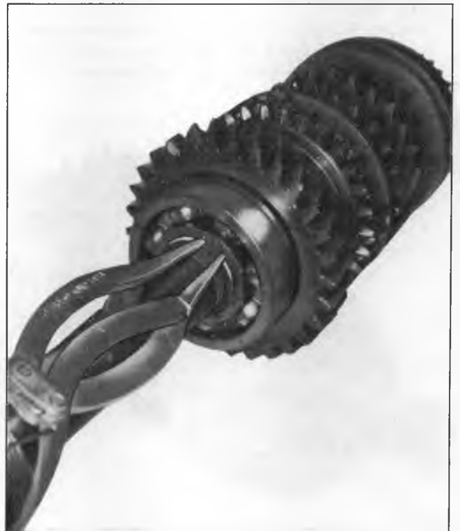
Fig. 8X--Third and Fourth Synchronizer Snap Ring
