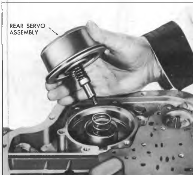
Fig. 148T--Installing Rear Servo Assembly
