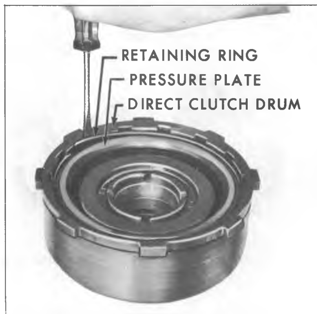
Fig. 72M--Removing Direct Clutch Pressure Plate
