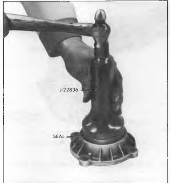
Fig. 16C--Installing Front Output Bearing Retainer Seal
