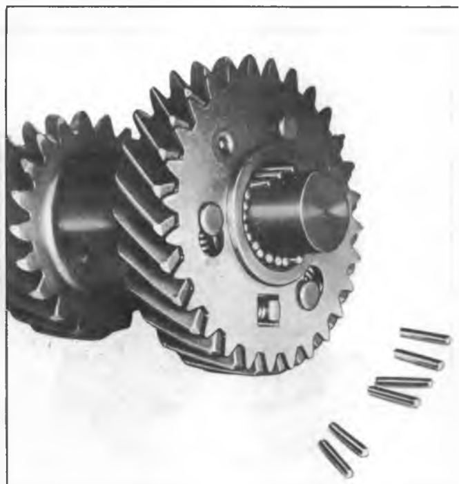
Fig. 23X—Loading Countergear Bearings
