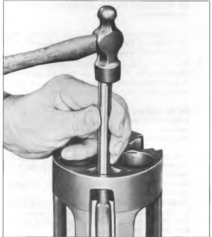
Fig. 18—Unseating Discharge Crossover Tube
