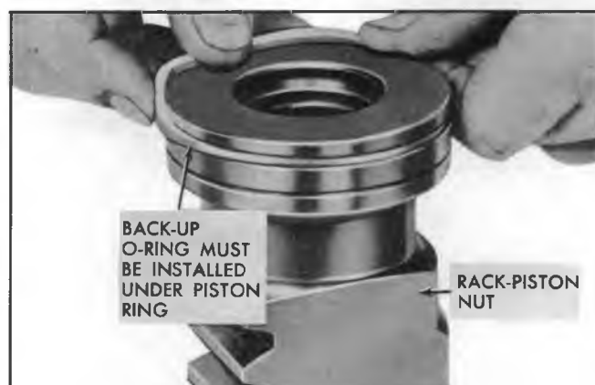
Fig. 47--Installing Ring on Rack-Piston
