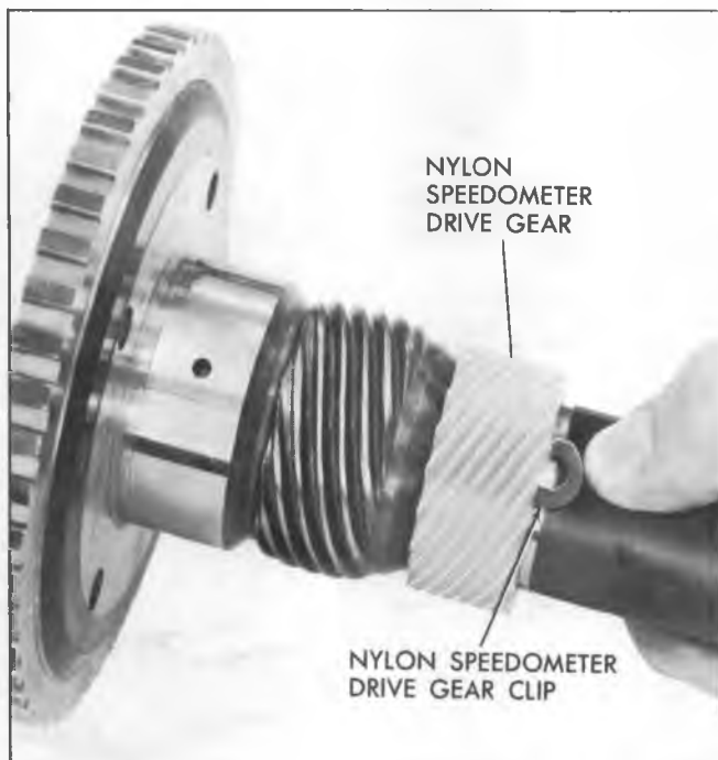
Fig. 46T-Removing Speedometer Drive Gear
