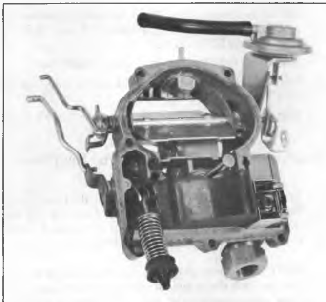
Fig. V6--Air Horn Assembly--Parts Location
