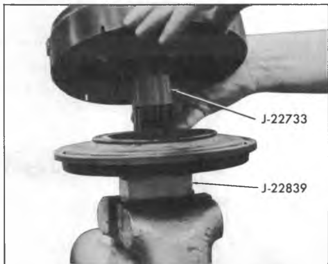
Fig. 6C--Installing Seal Protector Using Tools J-22733 and J-22839
