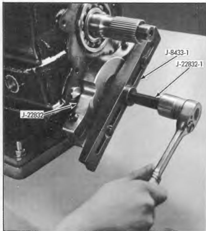
Fig. 3Q—Removing Countergear Rear Bearing
