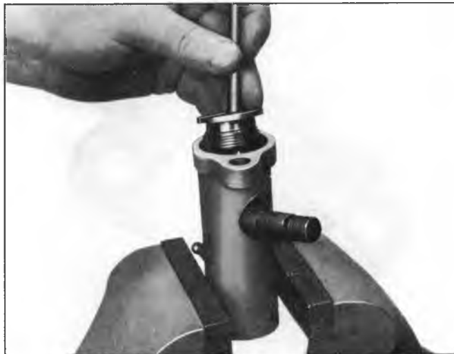
Fig. 72--Replacing Adjuster Plug and Shaft
