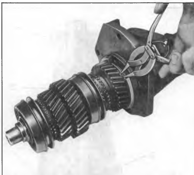
Fig. 3G—Removing Rear Extension From Mainshaft
