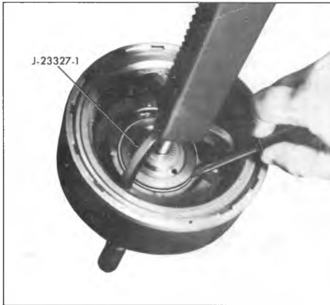
Fig. 82M--Compressing Forward Clutch Piston Return Seat
