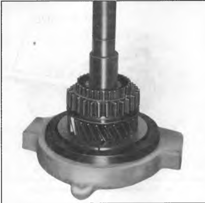
Fig. 13X—Removing 1-2 Synchronizer and Second Speed Gear
