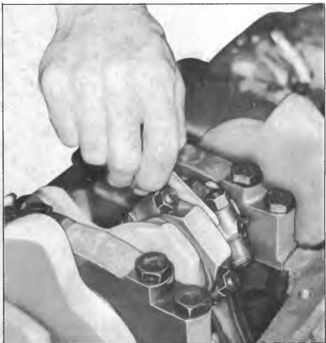
Fig. 47--Measuring Connecting Rod Side Clearance (V8)
