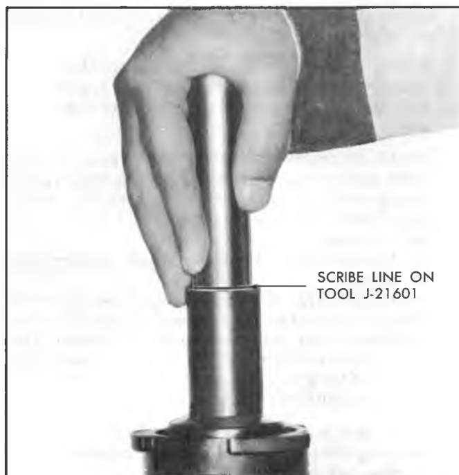
Fig. 7A—Installing Air Valve and Retainer
