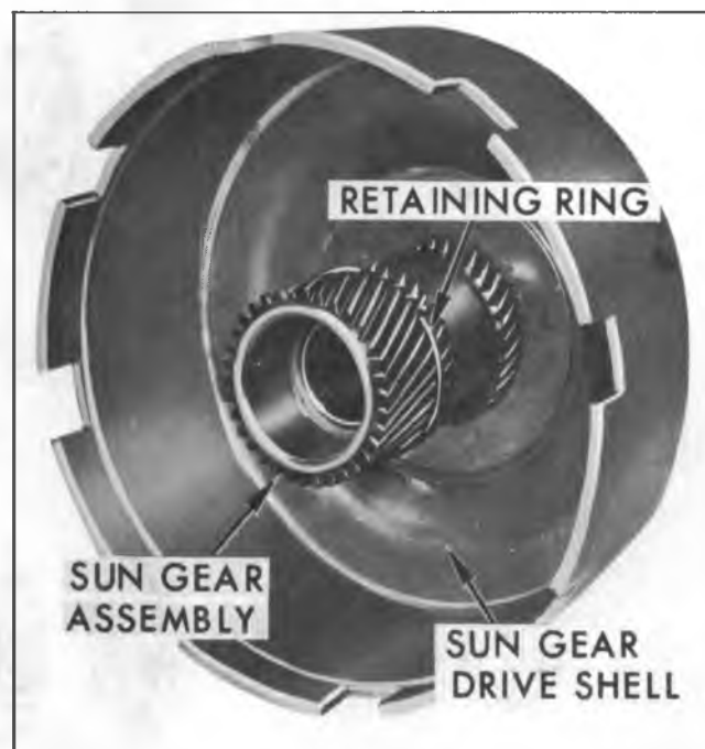
Fig. 90M—Removing Sun Gear to Drive Shell Front Steel Thrust Washer
