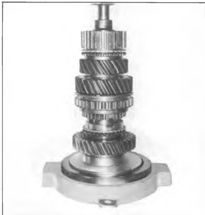
Fig. 22X—Installing Rear Bearing
