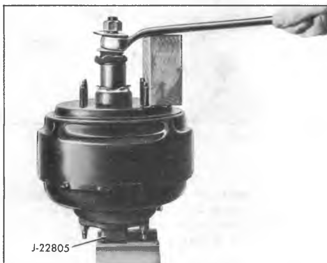
Fig. 3C—Removing Valve Rod, Air Silencer and Filter
