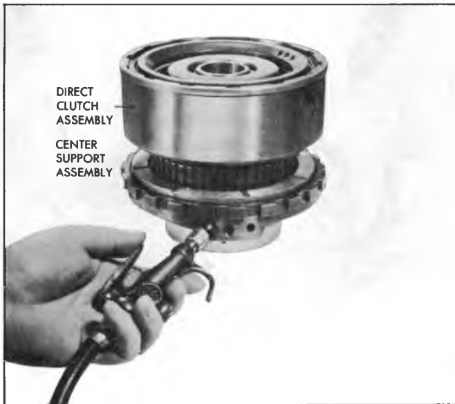
Fig. 97T--Air Checking Direct Clutch Assembly
