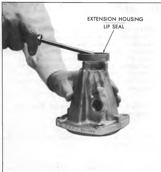
Fig. 5M--Removing Extension Housing Lip Seal
