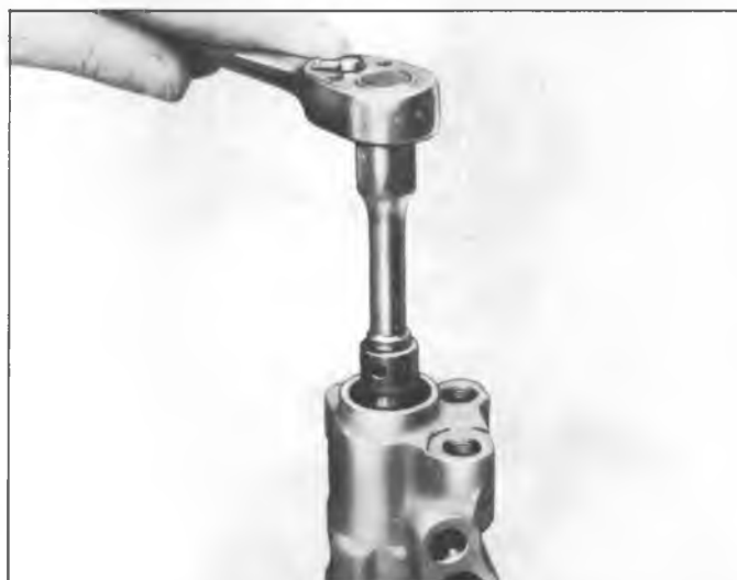
Fig. 64—Removing Adjusting Nut
