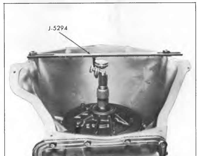
Fig. 108M--Checking End Play for Proper Thrust Washer Selection
