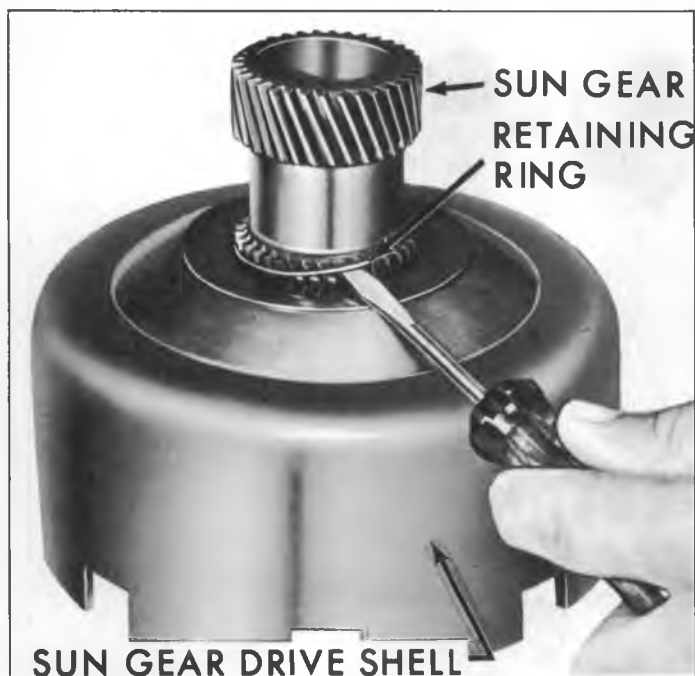
Fig. 88M—Removing Sun Gear Drive Shell Rear Retaining Ring
