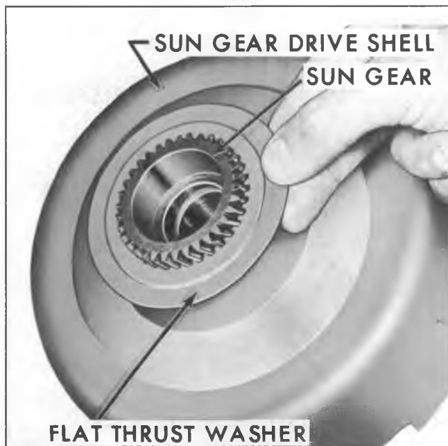
Fig. 89M—Removing Sun Gear to Drive Shell Rear Steel Thrust Washer
