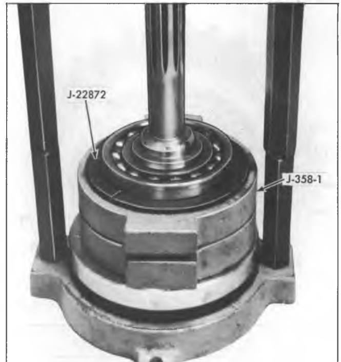
Fig. 10Q--Removing Clutch Gear Bearing
