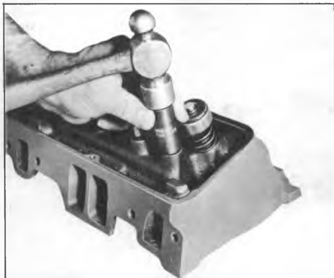
Fig. 21--Installing Rocker Arm Stud (In-Line and "Small V8")
