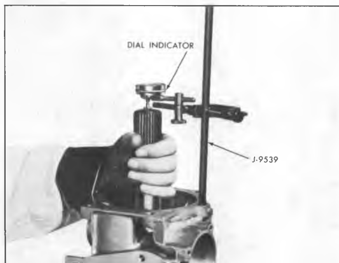
Fig. 32T--Checking Rear Unit End Play
