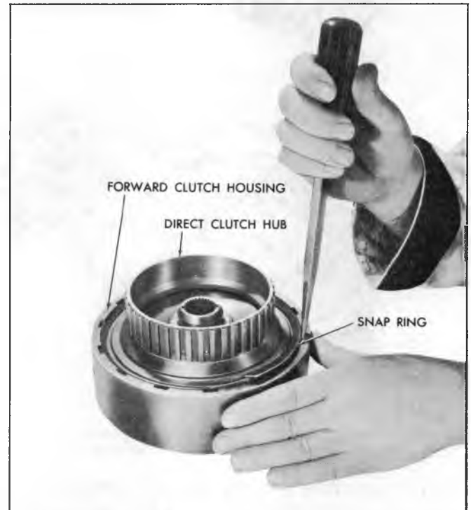
Fig. 77T—Installing Forward Clutch Housing to Direct Clutch Hub Snap Ring
