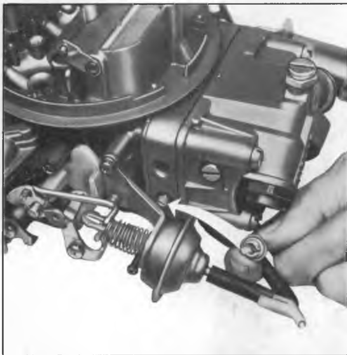
Fig. S-2 Holley Carburetor Idle Mixture Needle Limiter Caps
