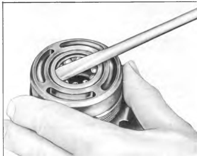
Fig. 7—Removing Lower Bearing Retainer—Except Corvette
