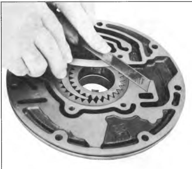
Fig. 65T--Checking Pump Body Face to Gear Face Clearance
