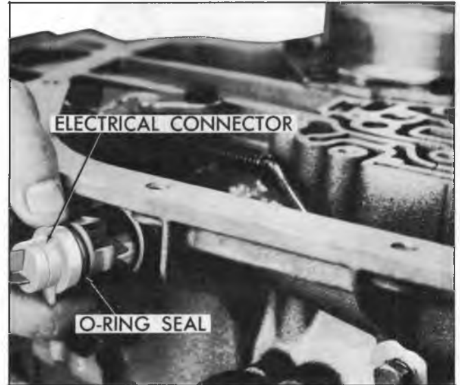
Fig. 145T--Installing Electrical Connector and "O" Ring Seal
