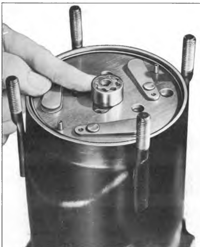
Fig. 15—Proper Oil Pump Gear Positioning
