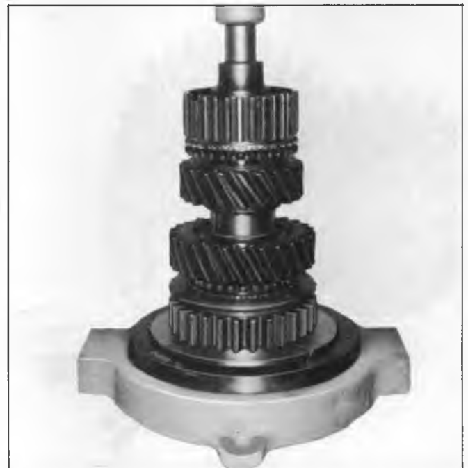
Fig. 21X—Installing 1-2 Synchronizer and Second Speed Gear
