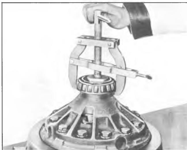
Fig. 11F--Differential Bearing Removal
