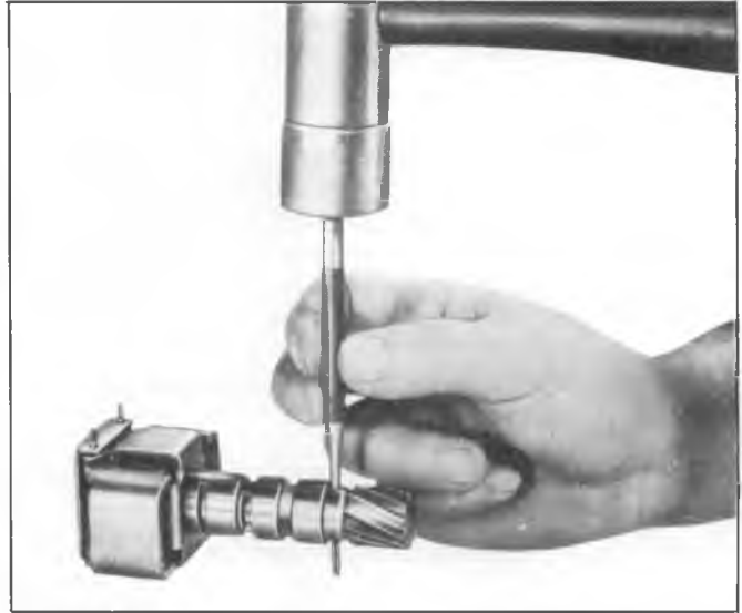
Fig. 49T--Removing Governor Gear Retaining Pin
