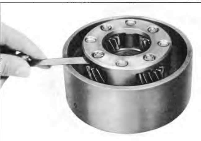
Fig. 105T--Checking Pinions End Play
