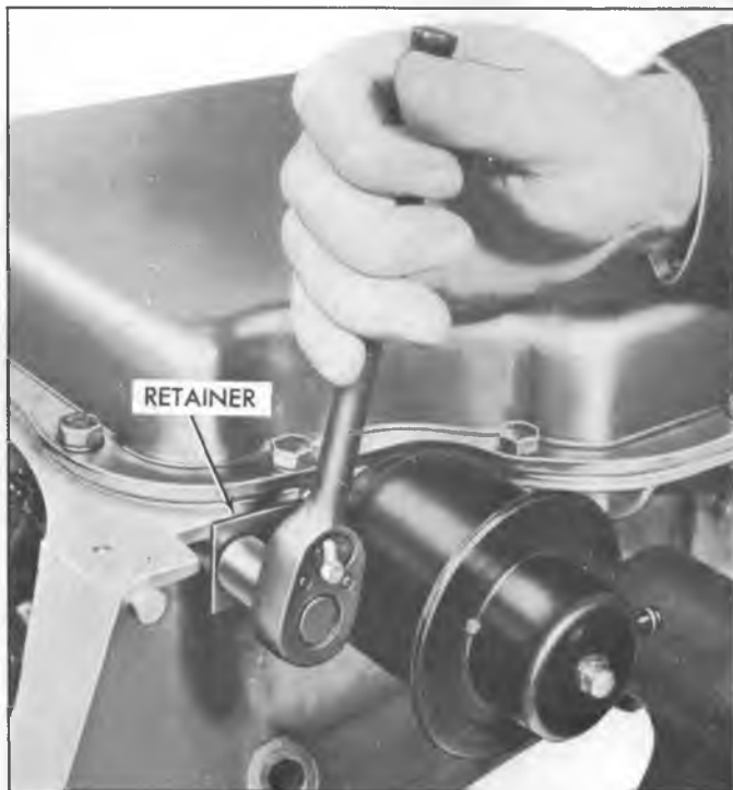
Fig. 3T--Removing Modulator Retainer
