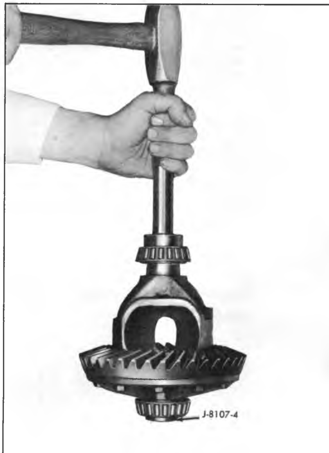
Fig. 3B-Differential Bearing Installation
