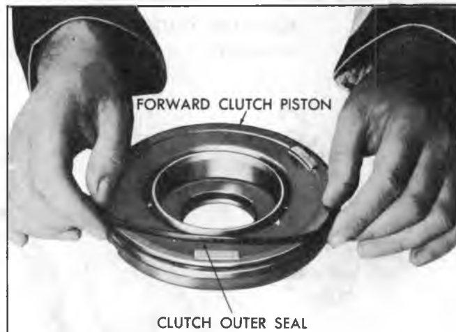
Fig. 71T--Removing Forward Clutch Piston Outer Seal
