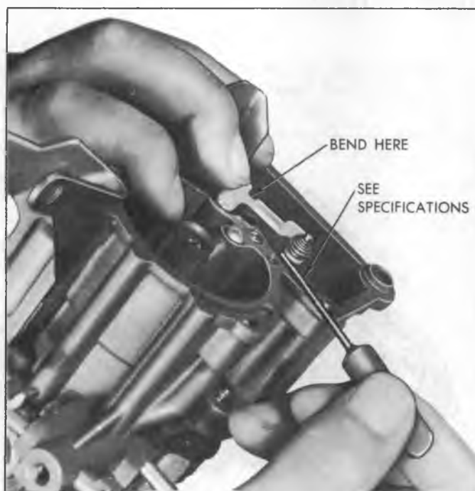
Fig. M5--Metering Rod Adjustment
