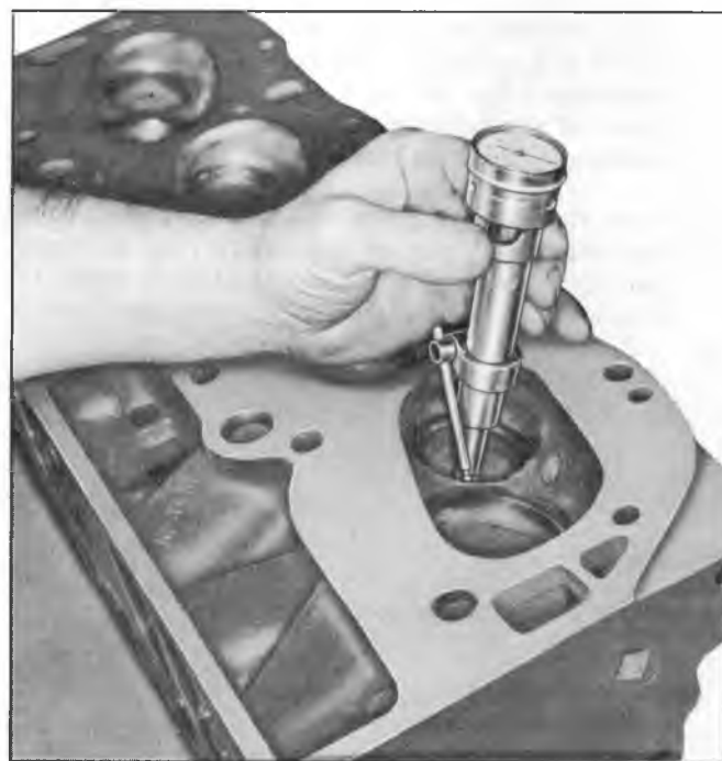
Fig. 24--Measuring Valve Seat Concentricity
