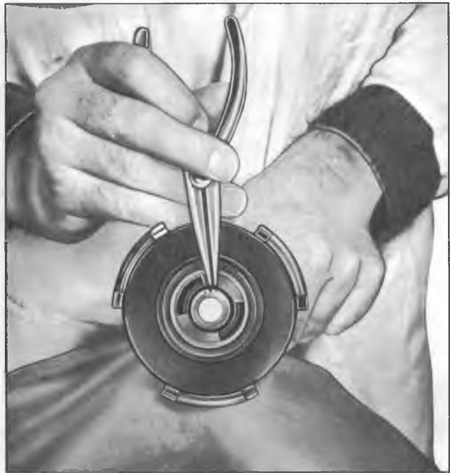
Fig. 10H--Removing Retaining Ring From Air Valve
