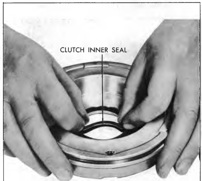
Fig. 85T--Installing Direct Clutch Inner Seal
