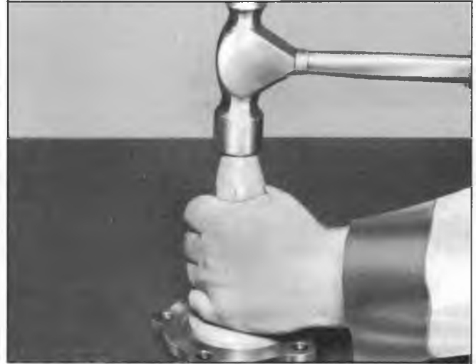
Fig. 7F--Pinion Oil Seal Installation (Typical)
