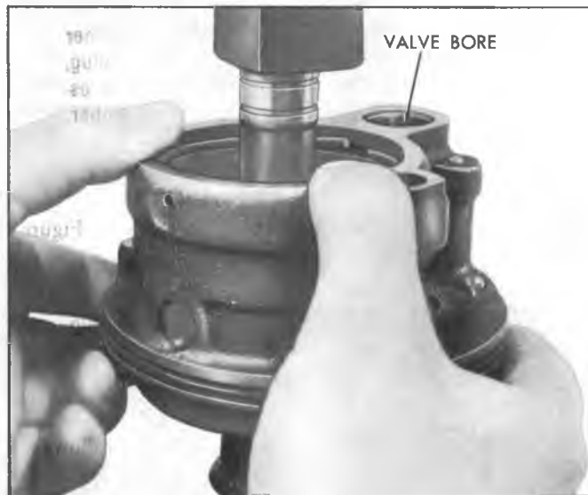
Fig. 29--Installing End Plate Retaining Ring
