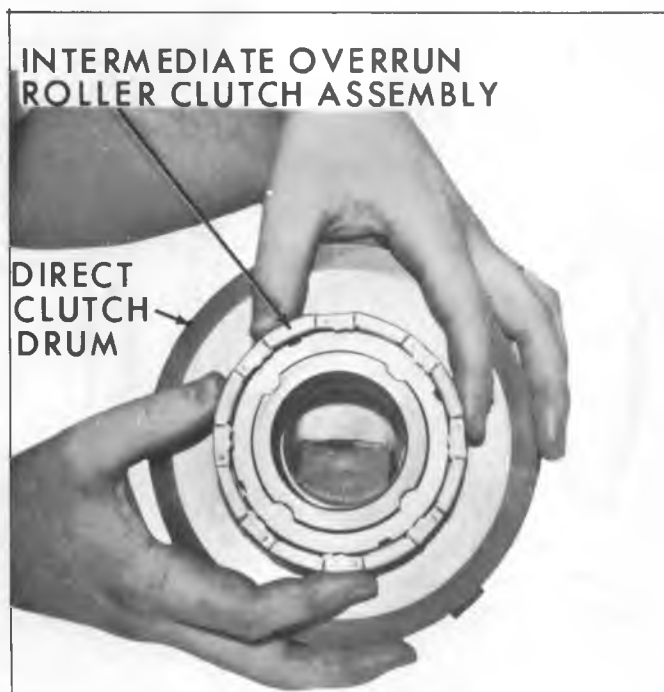
Fig. 70M--Removing Intermediate Overrun Roller Clutch
