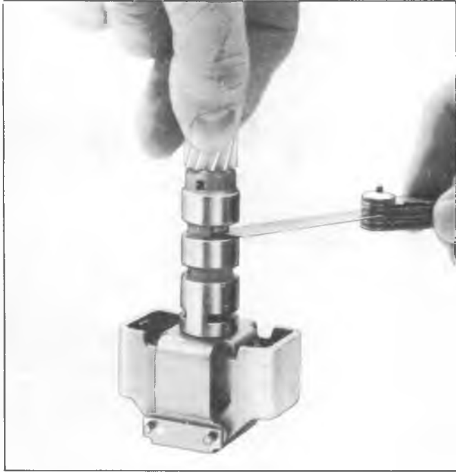
Fig. 48T-A--Checking Valve Opening With Weights Outward
