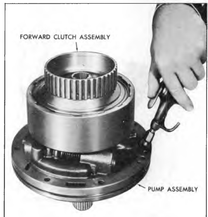
Fig. 78T—Air Checking Forward Clutch Assembly
