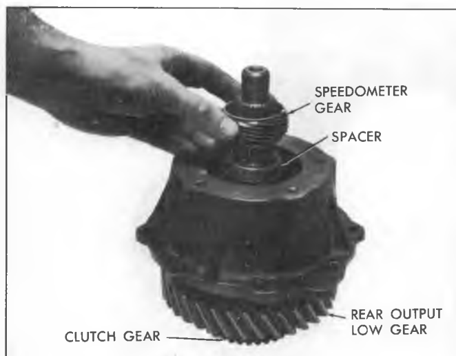
Fig. 18C—Installing Rear Output Shaft Spacer and Speedometer Gear
