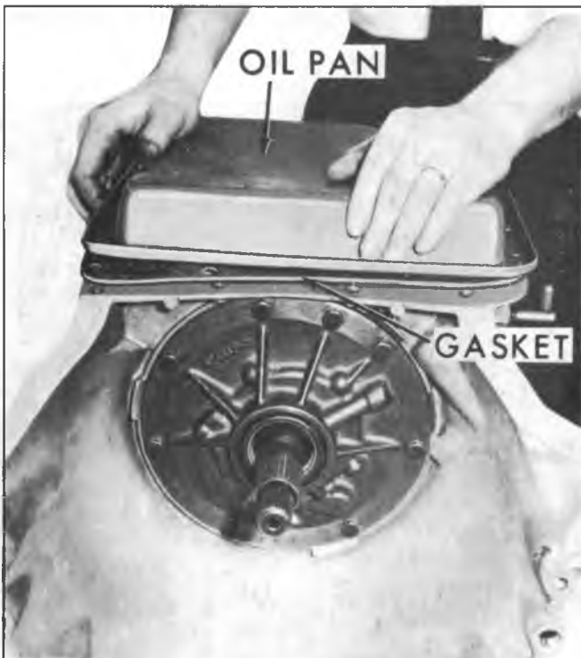
Fig. 10M--Removing Transmission Oil Pan
