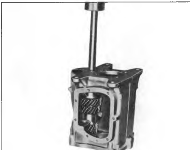
Fig. 8B—Removing Countershaft With J-22246
