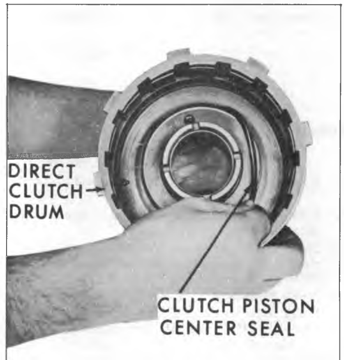
Fig. 76M--Removing Direct Clutch Piston Center Seal on Drum
