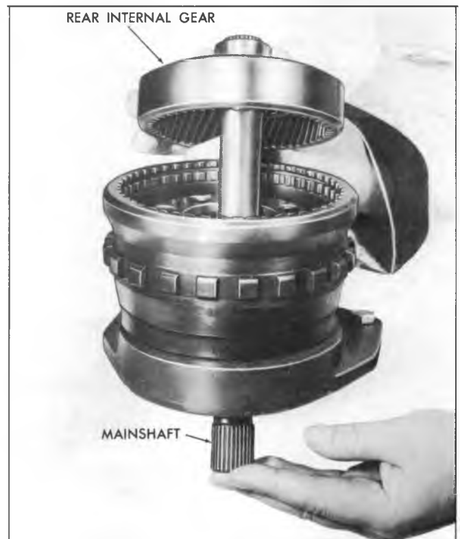
Fig. 44T--Removing Rear Internal Gear and Mainshaft
