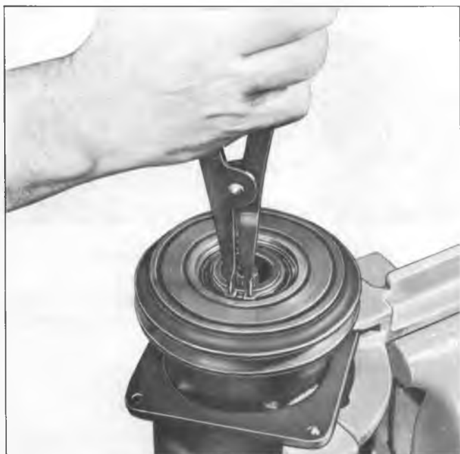
Fig. 6—Removing Pulley and Bearing Assembly Retainer Ring
