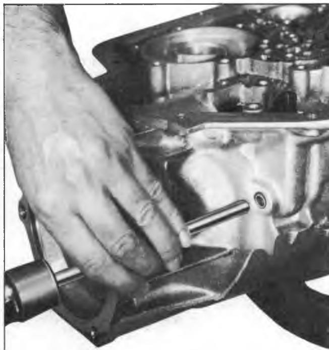
Fig. 127T--Installing Parking Pawl Shaft Cup Plug
