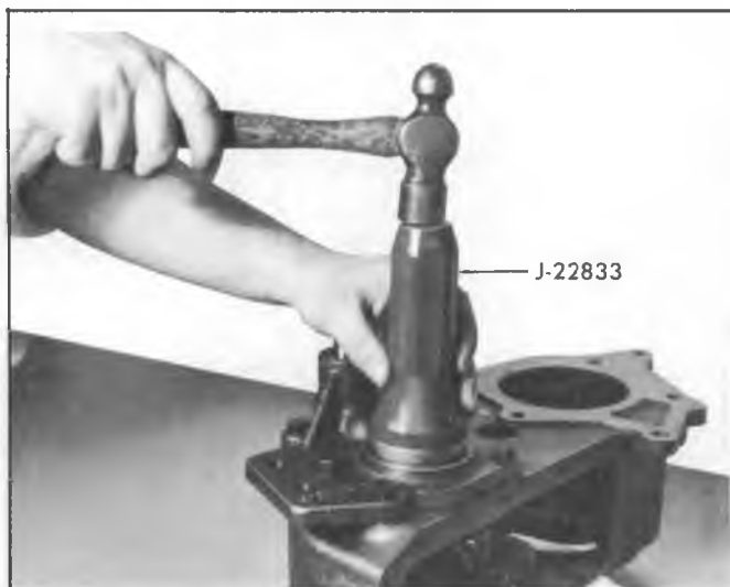
Fig. 15D—Installing Front Output Shaft Seal
