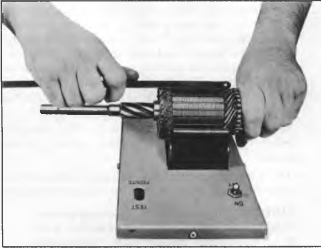
Fig. 4S--Armature Short Circuit Test
