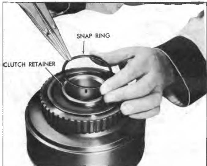
Fig. 95T-Installing Intermediate Clutch Retainer Snap Ring
