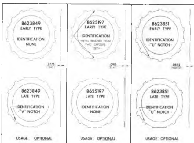
Fig. 76T—Forward Clutch Plate Identification
