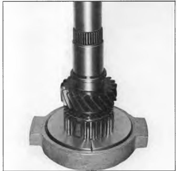
Fig. 20X—Installing 3-4 Synchronizer and Third Gear
