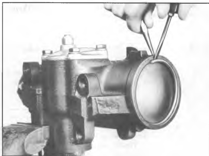
Fig. 32--Removing End Cover Retaining Ring
