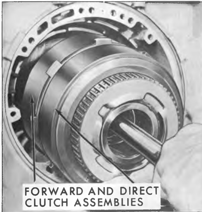
Fig. 33M--Removing Direct and Forward Clutch Assemblies
