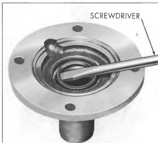
Fig. 17X--Removing Bearing Retainer Oil Seal
