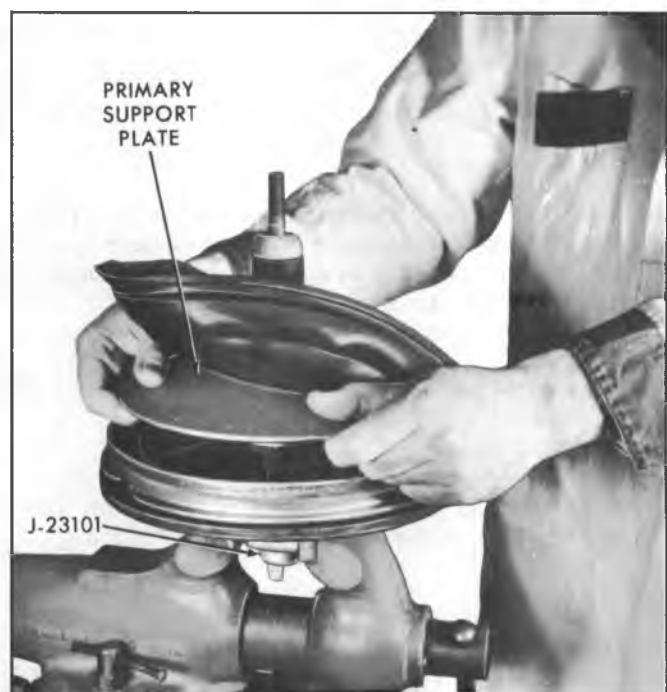
Fig. 5H—Locking or Unlocking Primary and Secondary Power Pistons
