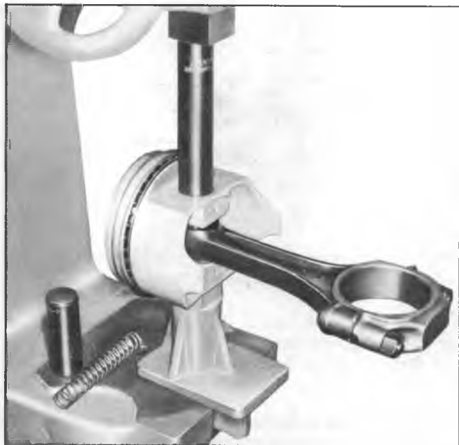
Fig. 52--Removing Piston Pin ("Mark IV V8")
