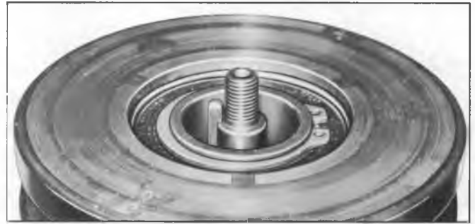
Fig. 4—Drive Plate Key Installed in Keyway
