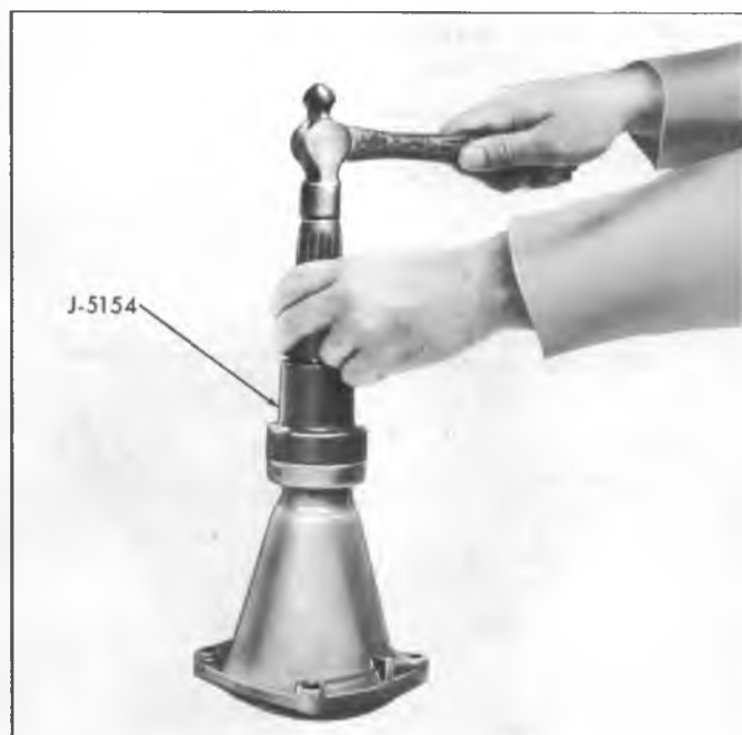
Fig. 109M—Installing Extension Housing Seal
