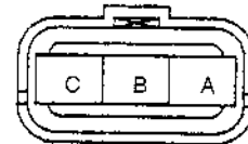
HARNESS SIDE CONNECTOR (VIEW FROM TERMINAL SIDE)
